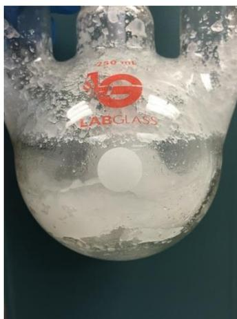
Figure 5.3. Polymerization result of SDS stabilized emulsion.
