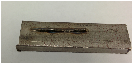
(a) First Deposit from Wheel Feeder System
