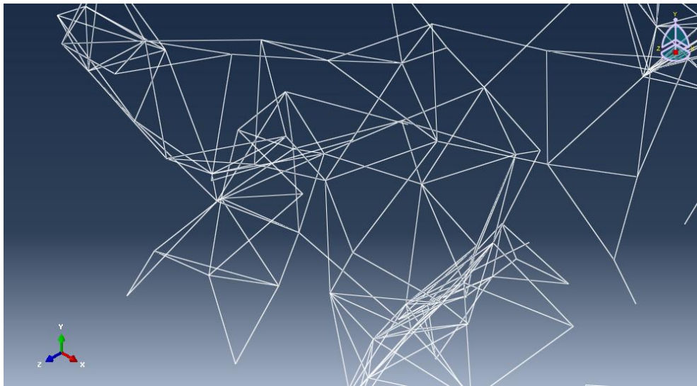
Figure 2.2. Finite Element Model for Aerogel Simulation. The white lines are beam elements that represent particle bonds. The centers of the particles lie on the intersection of these lines and are rigid nodes.
