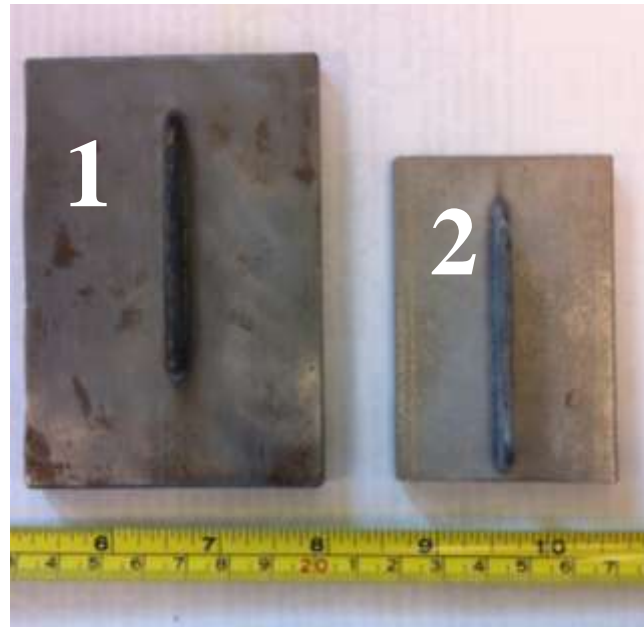
FIG. 10. DEPOSITS ON SUBSTRATES WITH A LARGE \xi_{sub} VALUE (1) AND A SMALL \xi_{sub} VALUE (2).
