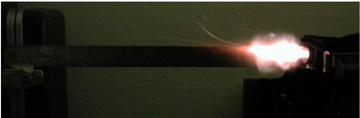
Figure 2.3. Lapua Palma case, 0.062" Flash Hole, Remington 7.5 Primer. (7)
