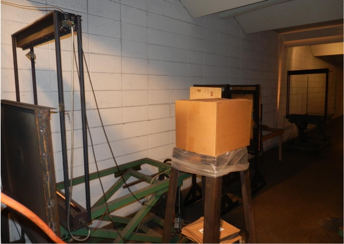
Figure 3.26. Velocity screens in range room at Fiocchi of America.
