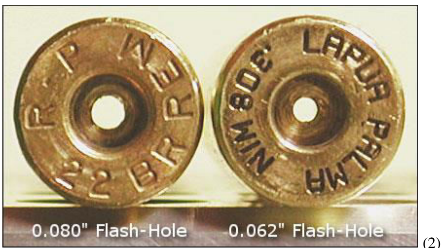
Figure 2.1. .308 Remington BR brass and .308 Lapua Palma brass flash hole comparison.
