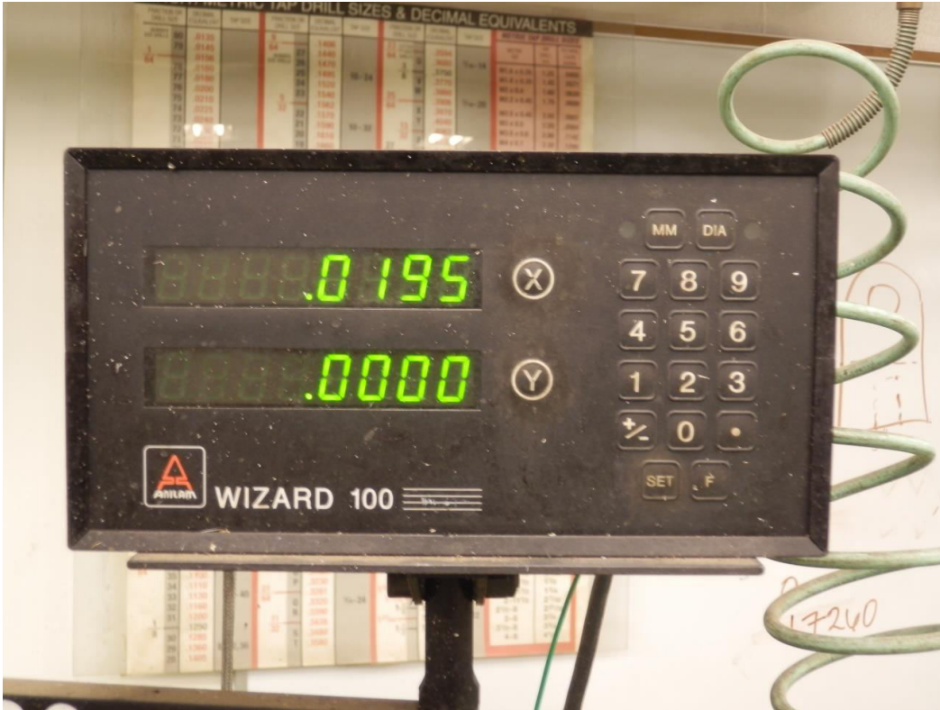
Figure 3.7. Drill offset 0.0195in (0.5mm).
