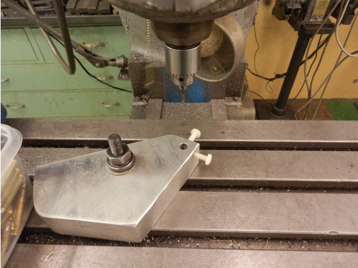
Figure 3.6. Anchored down aluminum block ready for drilling.
