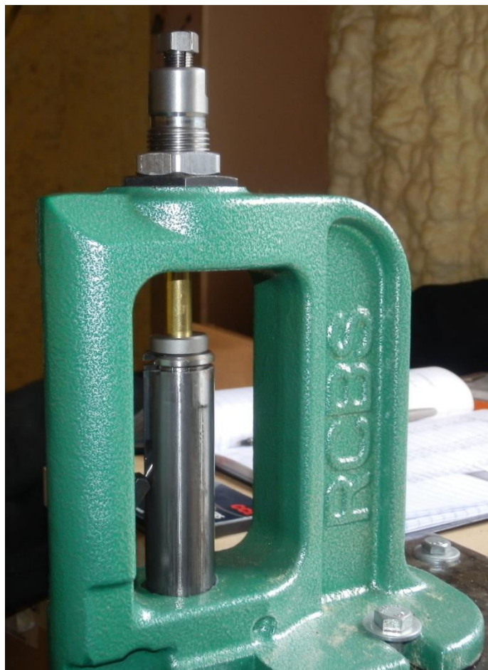
Figure 3.13. Case entering sizing die.
