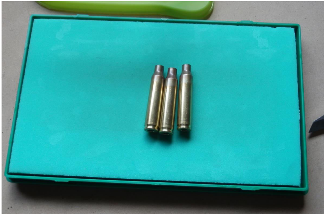
Figure 3.11. .223 cases on grease pad.
