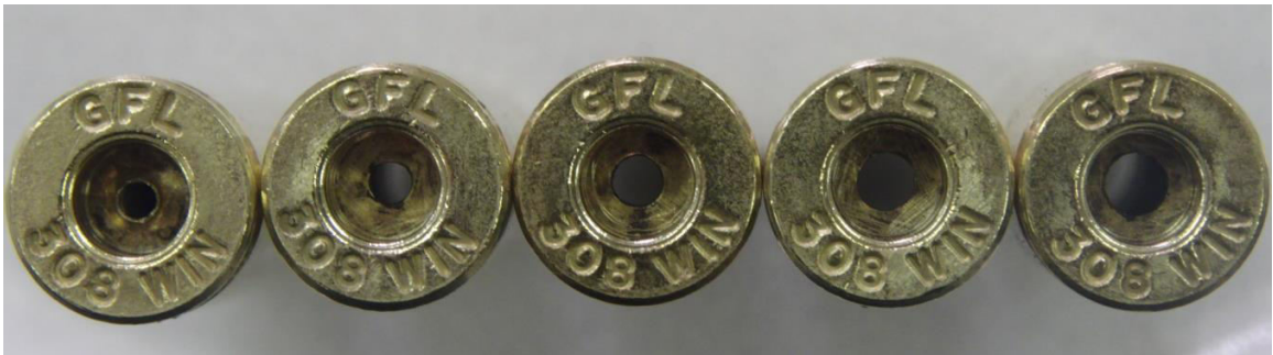
Figure 1.4. Left to right, 1.4mm, 2.0mm, 2.4mm, 2.8mm, 3.0mm flash holes drilled in .308 Winchester cases.
