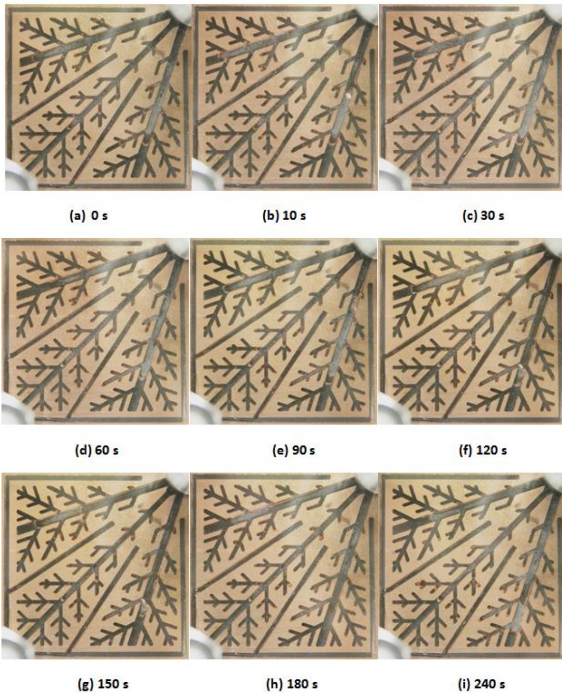
Figure 5.16 Time sequenced images showing water removal in bio-inspired channels at 0.35 V
