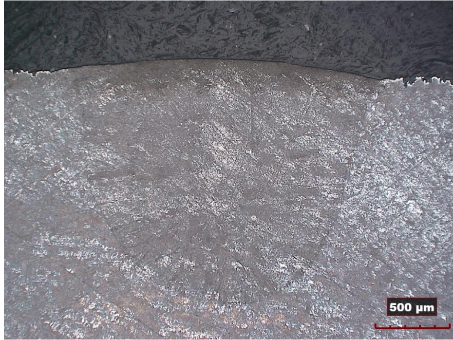
Figure 3-8 Microscopy of LSM sample at 0.7kW and 250mm/min travel speed
