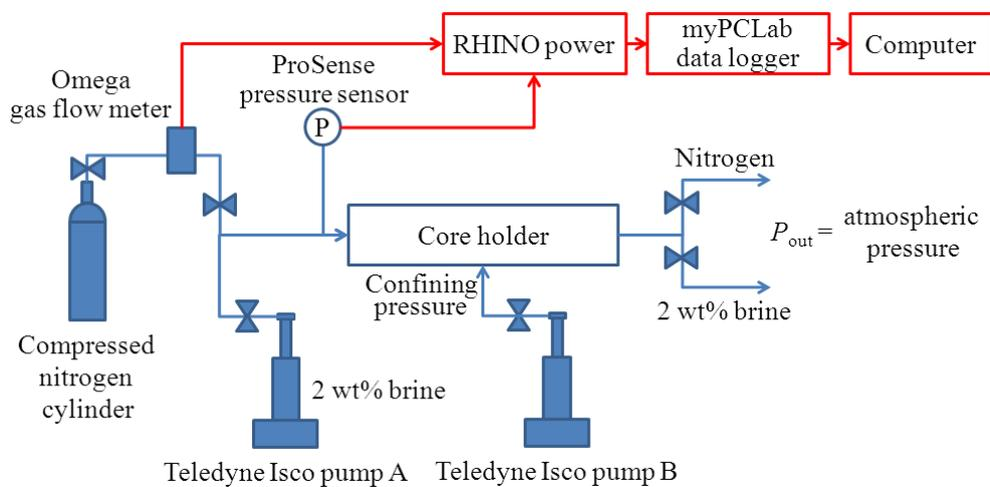
Figure 3.2. Diagram of Shale Fracture Model Experimental Setup
