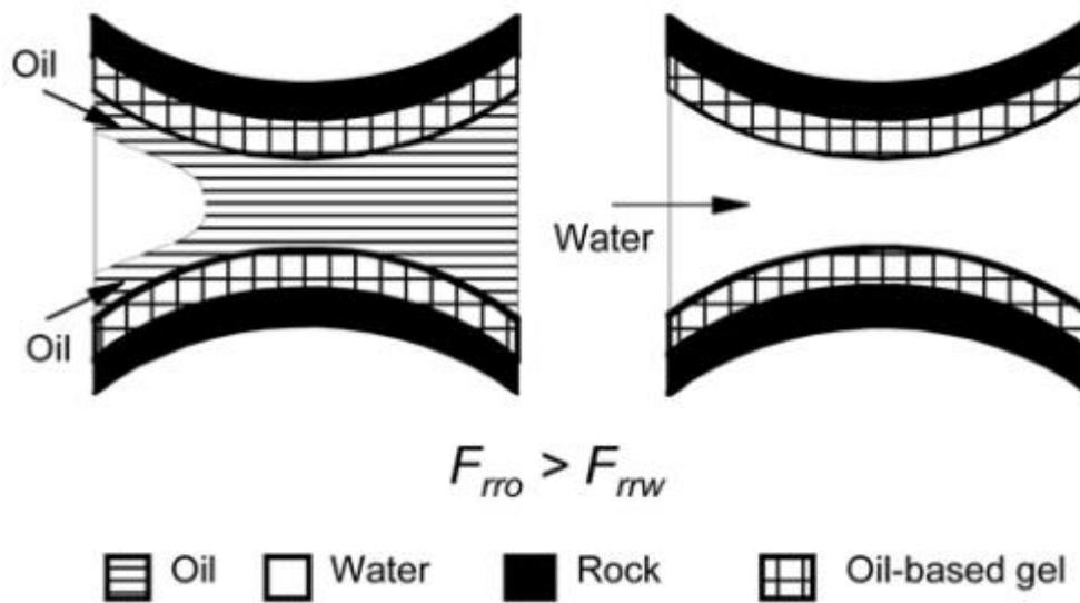
Figure 2.4. Wall-Effect Model; Oil Based Gel with Oil Wet Rock (Zaitoun et al 1998)
