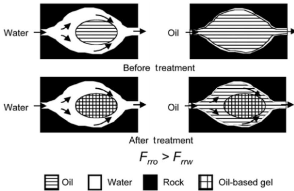
Figure 2.6. Gel-Droplet Model; Oil-Based Gel with Water-Wet Rock (Nilsson et al 1998)
