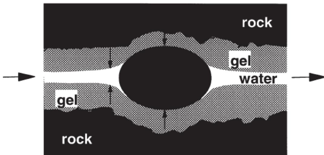
Figure 2.10. Balance between Capillary Forces and Gel Elasticity When Forcing Oil or Water through Water-Based Gel (Dawe And Zhang 1994)
