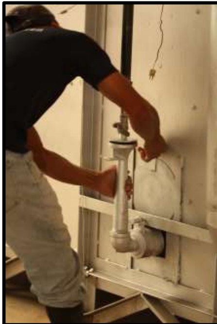
Figure 3.2: Closing the vents on the kiln.
