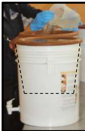
Figure 1.1: Typical CPF. A lid is placed on top to exclude additional contamination.
