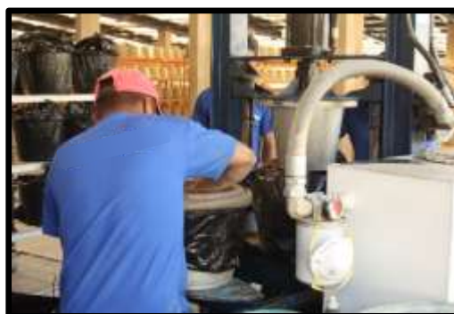
Figure 3.1: Shaping a CPF with a mechanical press.
