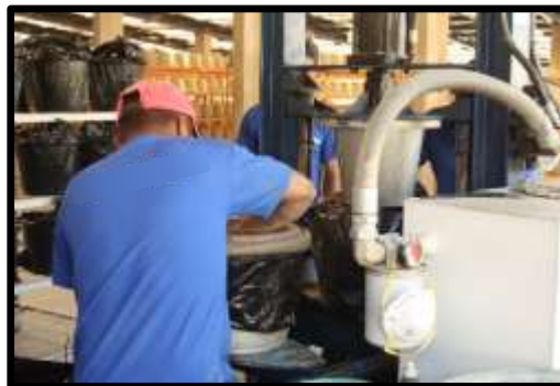
Figure 3.1: Shaping a CPF with a mechanical press.
