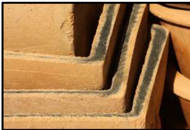
Figure 1.2: Carbon remnants in CPF cross sections.
