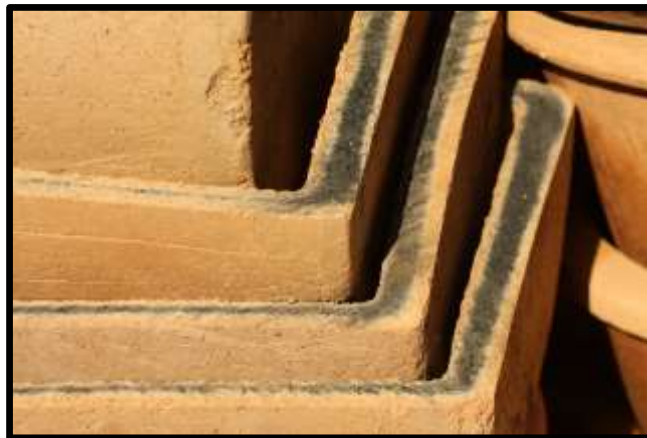
Figure 1.2: Carbon remnants in CPF cross sections.
