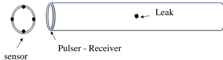
Figure 3.8. Leak Location And Sensors Configuration At The End Of Pipeline
