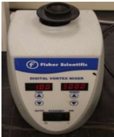
Figure 3.2. The digital mixer was used to mix the graduated tubes to obtain an emulsion phase
