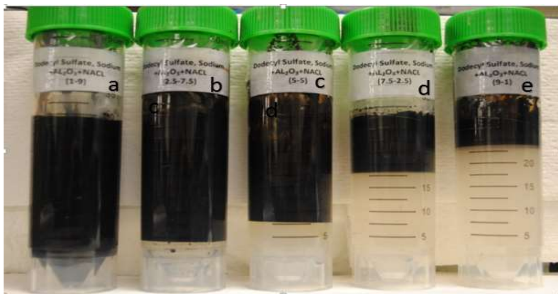
Figure 4.8. The results after SDS were combined with \text{Al}_2\text{O}_3 at 25^\circ\text{C} (24 hours). From left to right: 1:9, 2.5:7.5, 5:5, 7.5:2.5, and 9:1.
