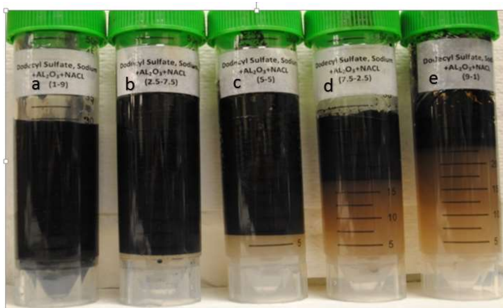
Figure 4.7. The results after SDS was combined with Al 2 O 3 at 25°C (four hours)
