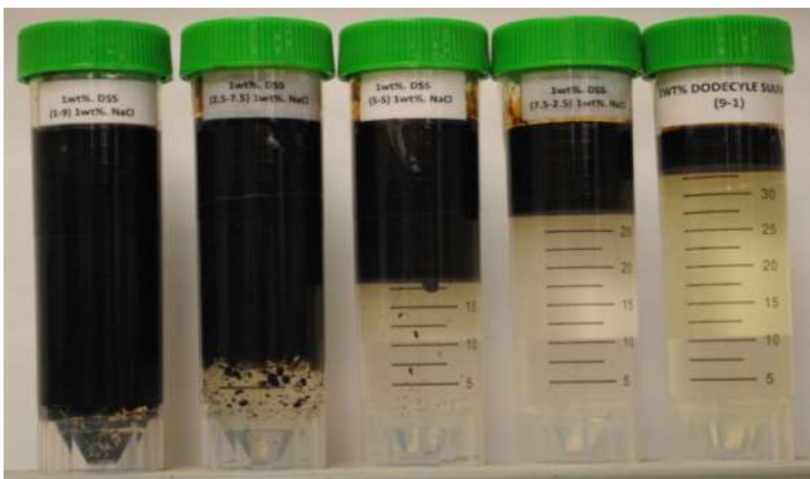
Figure 4.3. Unstable emulsion results of SDS at 25°C. From left to right: 1:9, 2.5:7.5, 5:5, and 7.5:2.5, 9:1
