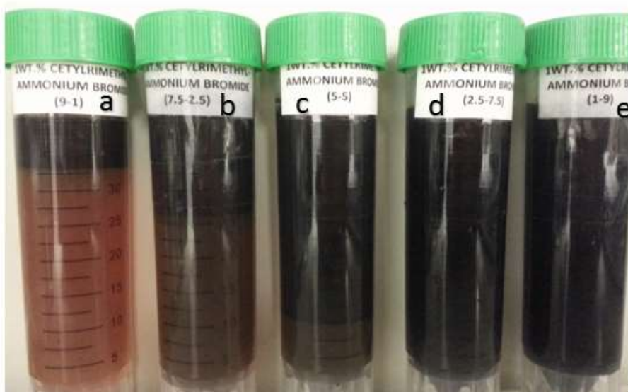
Figure 4.4. The results of CTABs immersed in A-Hauser (1) crude oil. From left to right: (9:1, 7.5:2.5, 5:5, and 2.5:7.5, 9:1)
