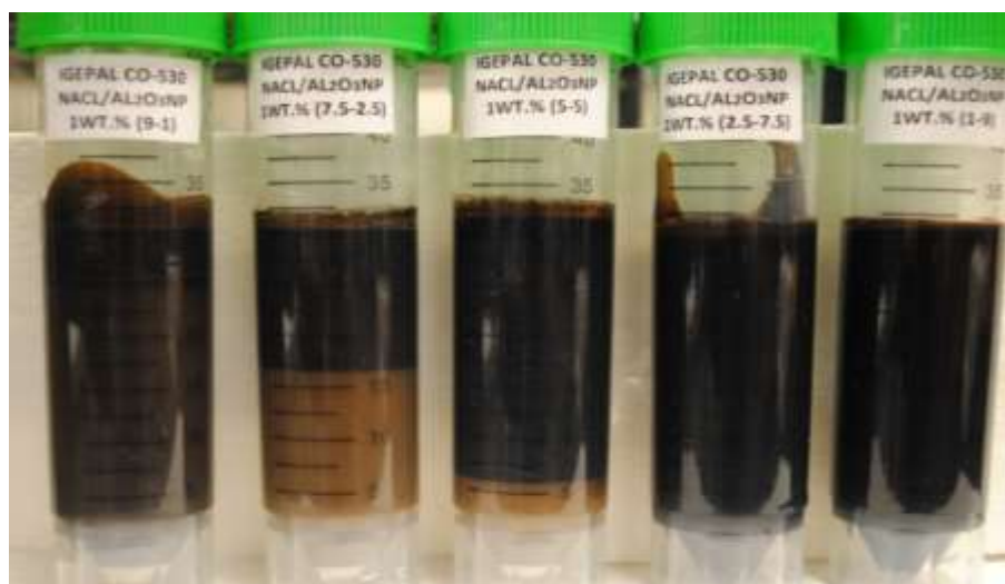
Figure 4.5. The results after IGEPAL CO-530 was combined with Al 2 O 3 at 25°C (24 hours)
