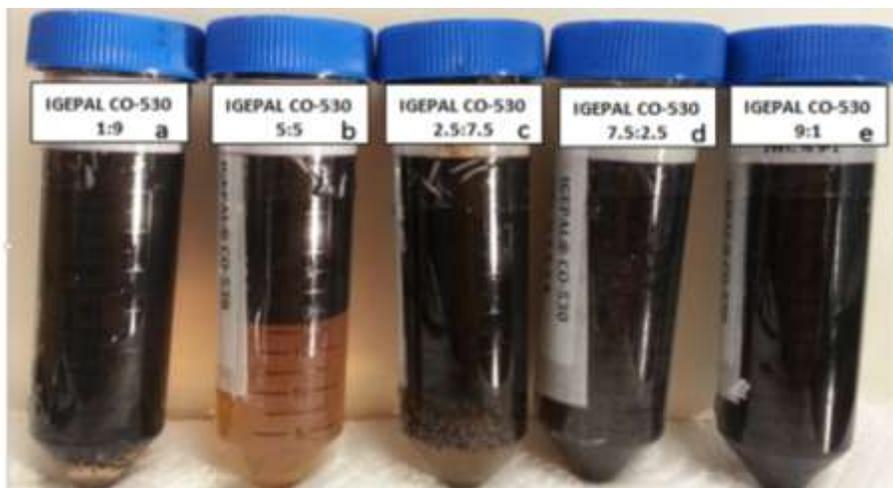
Figure 4.1. The result after IGEPAL CO-530 was combined with A-HAUSER (1) at 25°C
