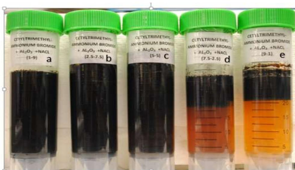
Figure 4.9. The results after CTAB was combined with  $\text{Al}_2\text{O}_3$  at  $25^\circ\text{C}$  (24 hours)
