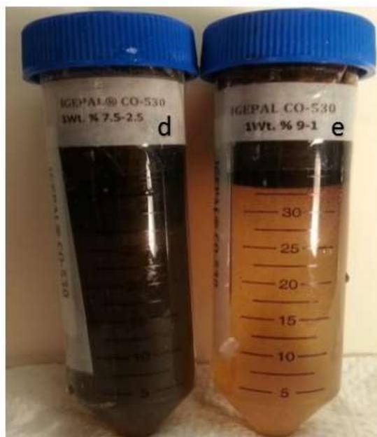
Figure 4.2. The result of ratio 7.5:2.5, and 9:1 water to oil after the temperature increased to 40°C
