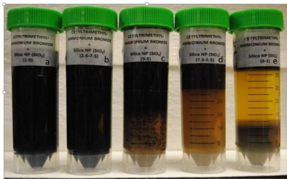
Figure 4.12. The results of adding  $\text{SiO}_2$  to CTAB at  $25^\circ\text{C}$  (24 hours)
