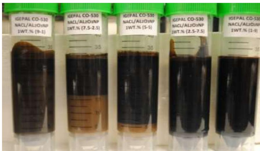
Figure 4.5. The results after IGEPAL CO-530 was combined with Al<sub>2</sub>O<sub>3</sub> at 25°C (24 hours)
