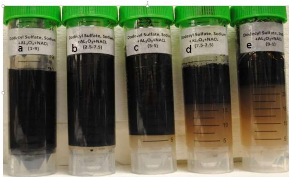
Figure 4.7. The results after SDS was combined with Al<sub>2</sub>O<sub>3</sub> at 25°C (four hours)
