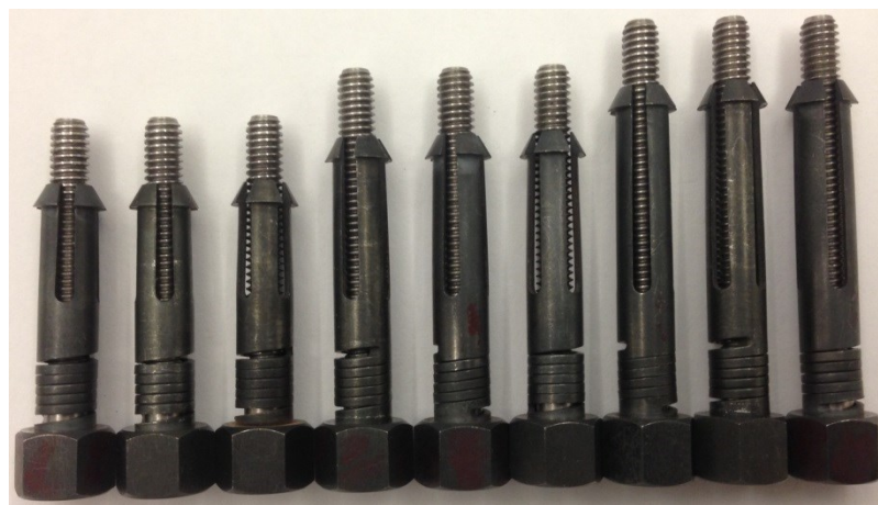
Figure 5.3. Working of the fastener – flexible finger expanded and spring compressed
