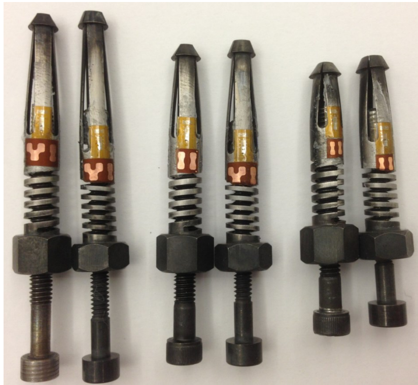
Figure 7.5. Temporary fasteners with bonded strain gage and terminals
