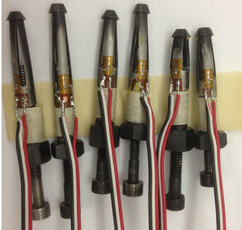
Figure 7.6. Wires soldered to the strain gages and terminals
