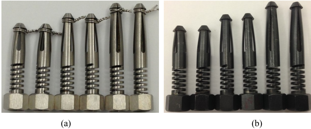
Figure 5.2. Fastener heat treatment: (a) fasteners held by steel wires and (b) fasteners after heat treatment
