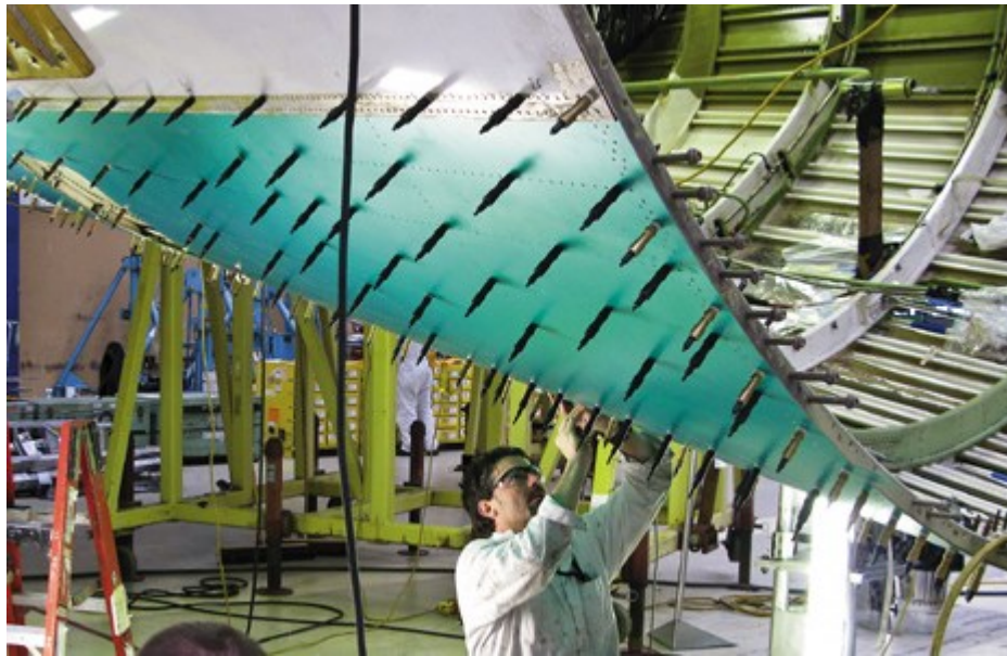
Figure 1.1. Temporary fasteners that hold the skin in place for riveting [1]
