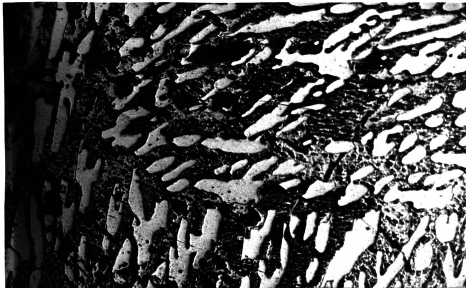
Figure 11. As-Cast, Induction Melted, 37.1 Wt.% (16.7 At.%) Ho Alloy. 3% Nital Etch. 200X. Phases Identified:  $\text{HoFe}_3$ ,  $\text{HoFe}_5$ ,  $\text{Ho}_2\text{Fe}_{17}$ .
