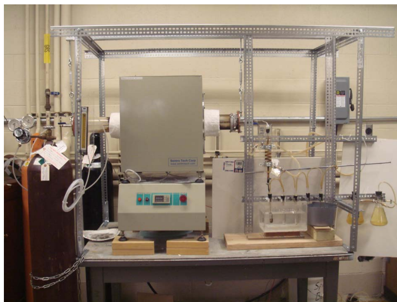
Figure 5.2. The Real Pyrolysis Experiment an Equipment Using Tube Furnace
