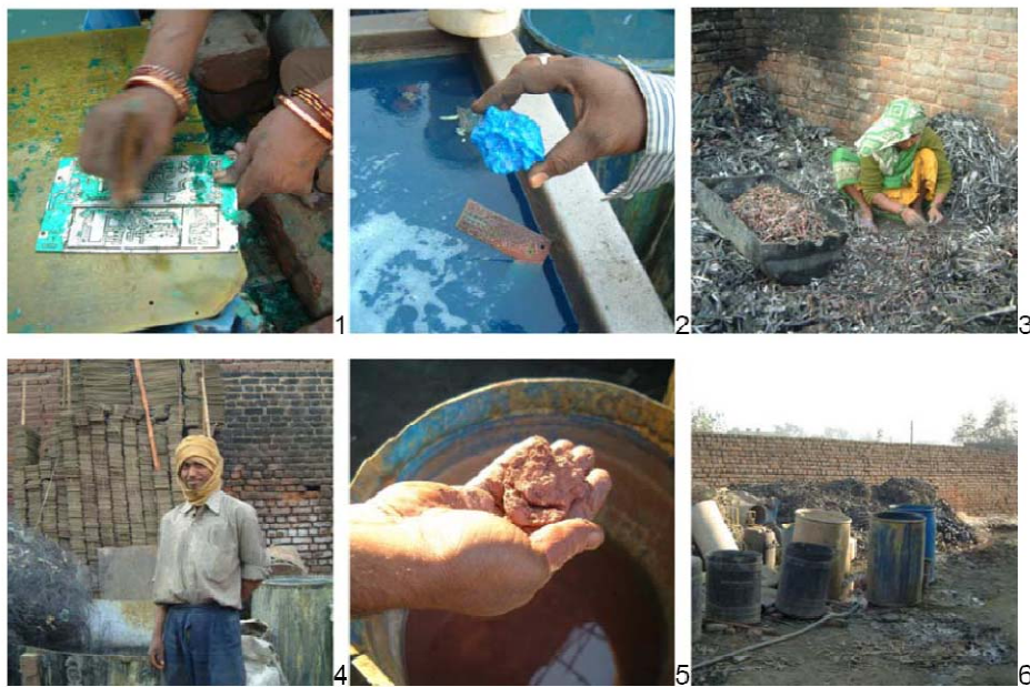
Figure 2.4. An Example of Low Quality Extraction of Copper from PWBs [1]
