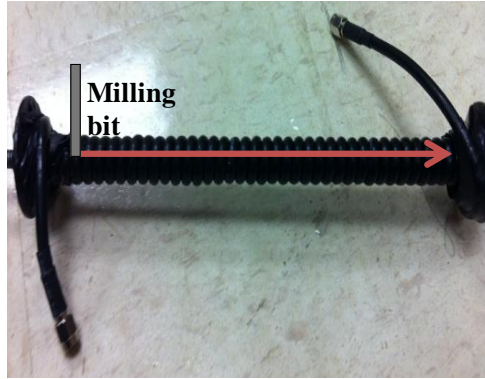
Figure 3.6. Image of a coiled coaxial cable resonator.
