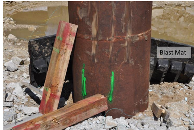
Figure 4-8. Pipe test general setup. The pipe was positioned vertically and covered with a blast mat to reduce hazards from pipe debris. The spray painted lines (green), on either end of the horizontal timber, were rough order of magnitude predictions of where the LSC liner fragments would impact the pipe.
