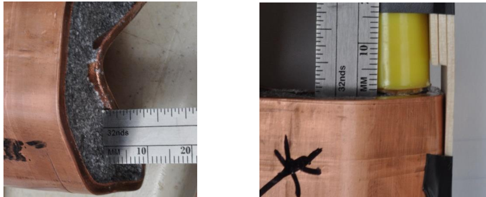
Figure 4-7. Explosive face disfiguration (left) extruded Pentolite used to match face disfigurations (right). The boosters were paired with the disfigurations to attempt to keep the length of explosives from the blasting cap to the LSC equivalent. This would ensure the LSC wings were initiated simultaneously.
