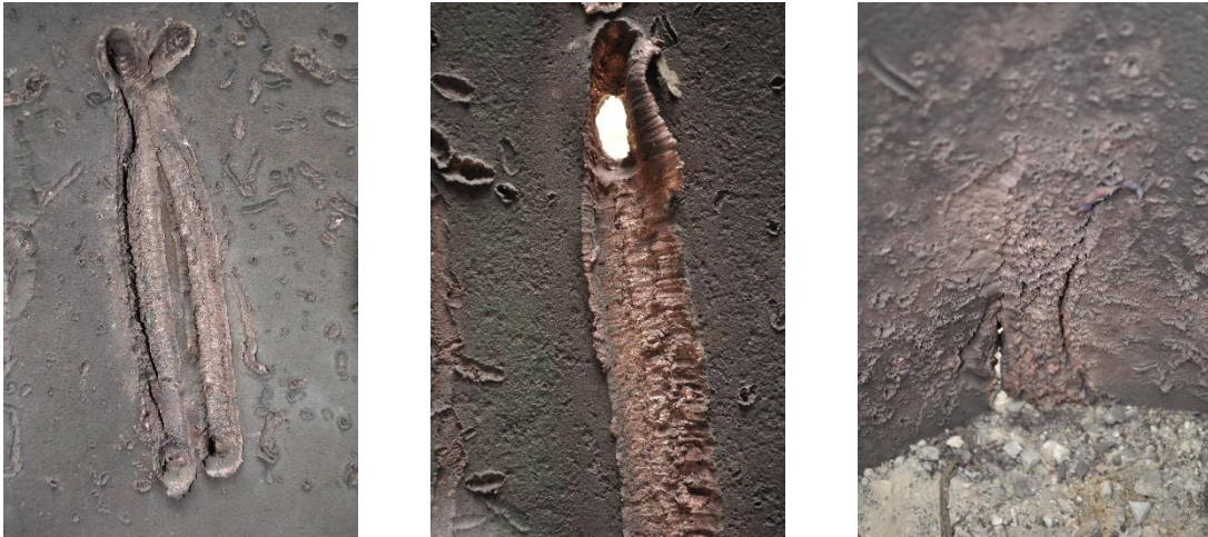
Figure 5-7. Top impact (left) unexpected perforation (center) debris cloud impact (right).
