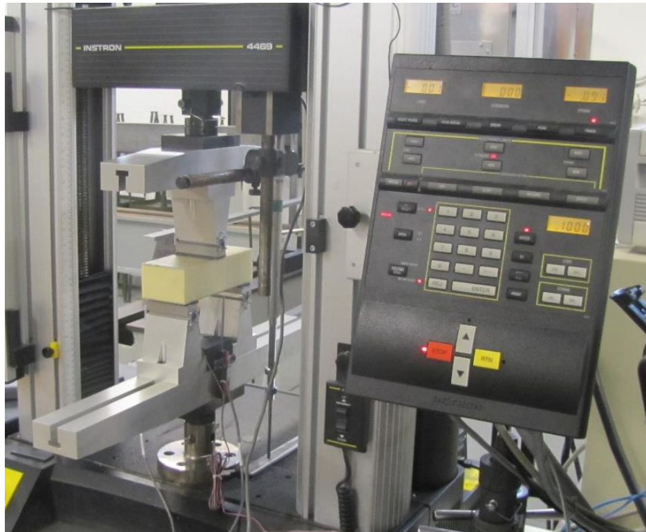
Figure 5.4: Test Setup Used for the Three Point Flexural Test
