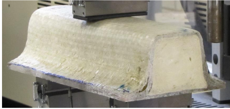
Figure 5.3: Three Point Flexural Test Specimen for Type 3
