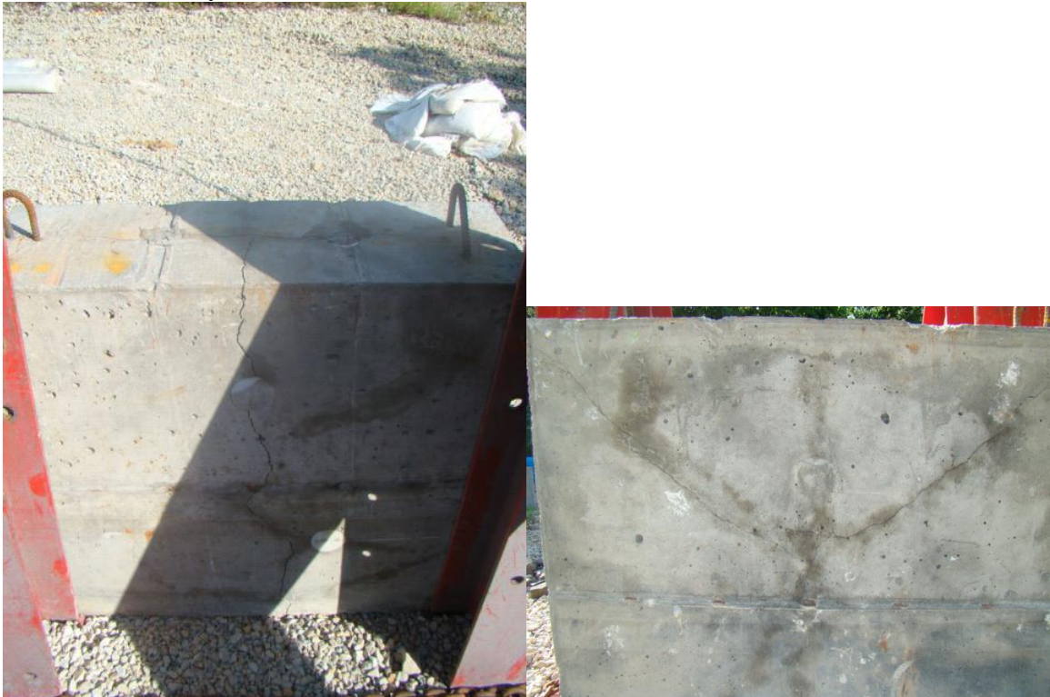
Barrier with cavity no LCFs
