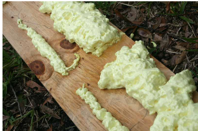
Figure 4.6 Canister and foam sprayed on board to observe expansion
