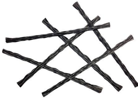
Figure 3.4 Long carbon fibers (Properma, 2014)
