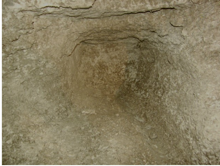
Figure 4.1. Typical Baseline Relief Hole Round (This picture of Test 10's results illustrates the uniform profile at the back of the cut, containing no craters or bootlegs)
