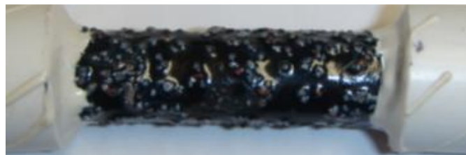
Fig.2. Sand particle-modified enamel coated steel bar.
