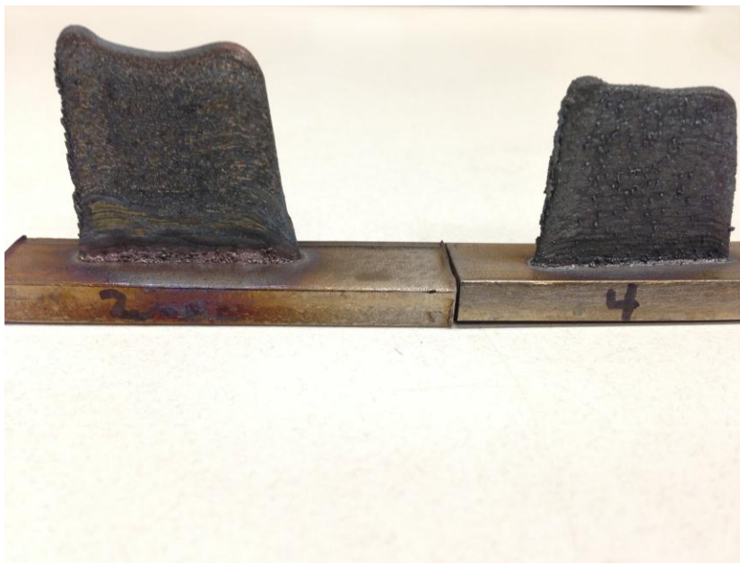
Figure 3.12. Comparison of Pre-Alloyed (Sample #2) and Mixed Elemental Powder (Sample #4) 430 SS Deposits
