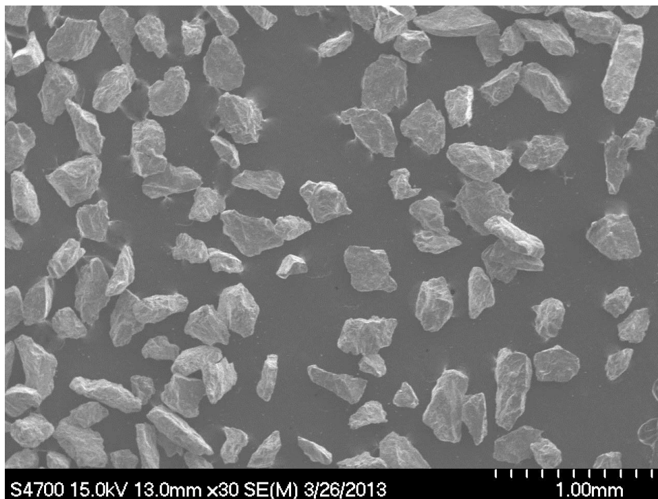
Figure 2.9. SEM Micrograph of Al/V Master Alloy Powder Particles
