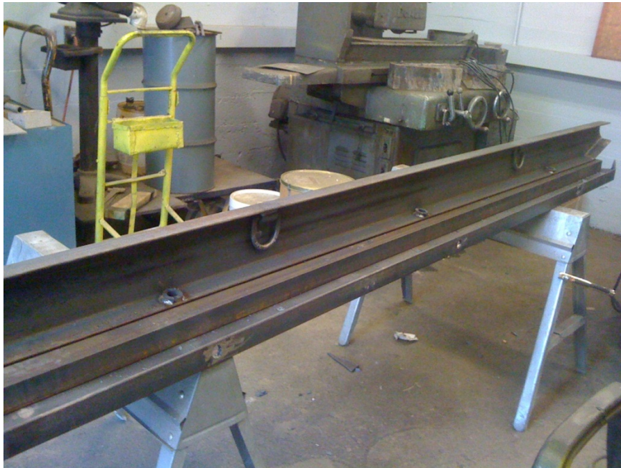
Figure 7.5. Side rails with D lashing rings
