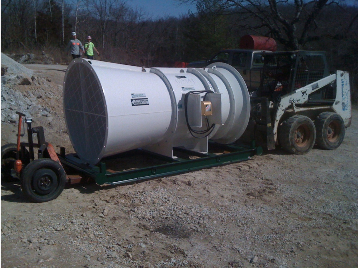
Figure 7.8. Booster fan transportation
