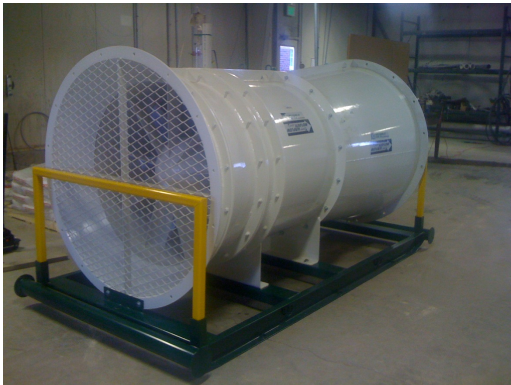
Figure 7.6. Completed skid with the mounted booster fan
