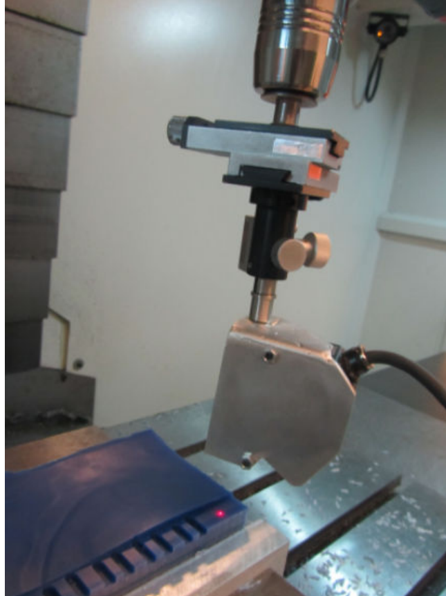
Figure 4.8 Measurement carried out along X axis using laser displacement sensor- Keyence LKG-5000.
