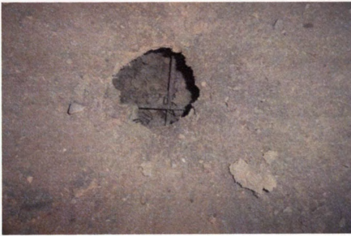
(c) Hole in the Compression Face
