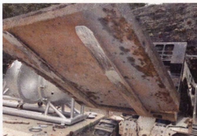
(g) Bulge in Tension Face
