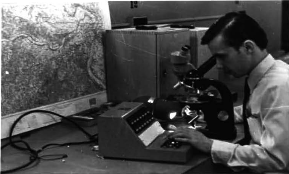
PICTURE 8. Performing the petrographic examination of aggregates with stereoscopic microscope, petrographic microscope, mechanical stage and electro-point counter.
