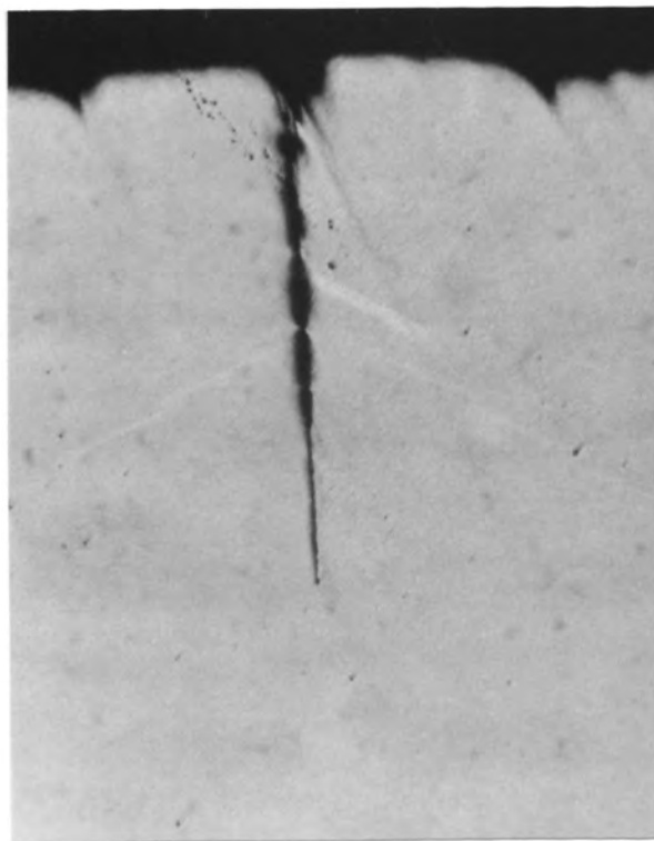
(c) 4200 cycles, 0.050 inch below the surface
