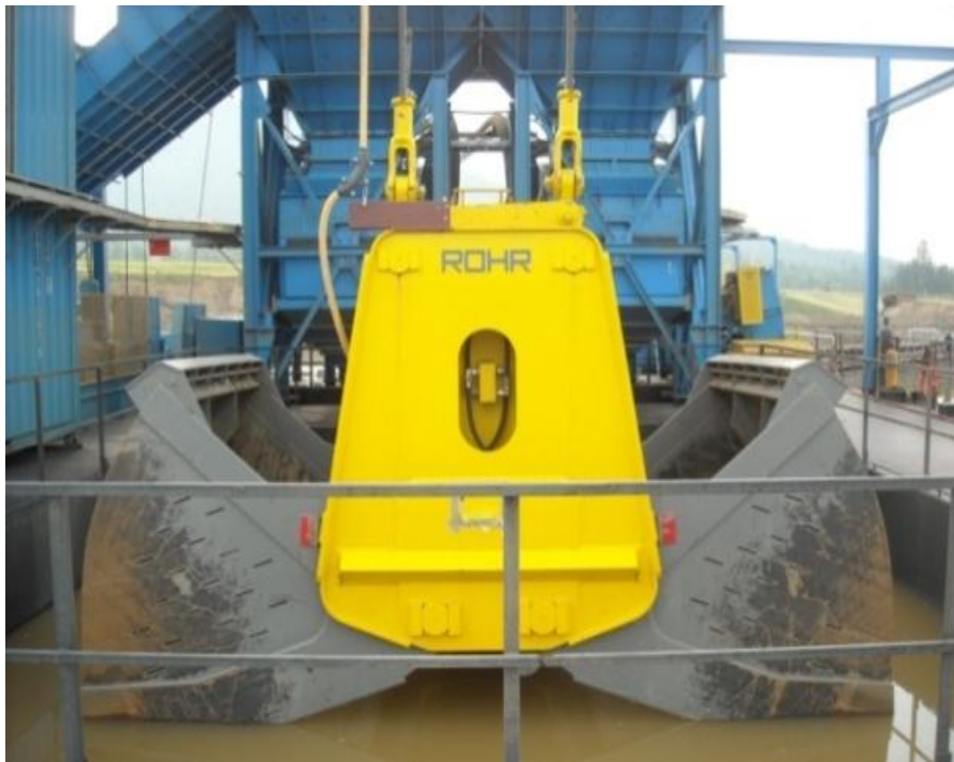
Figure 3.2 A Clamshell dredge being lowered under water
