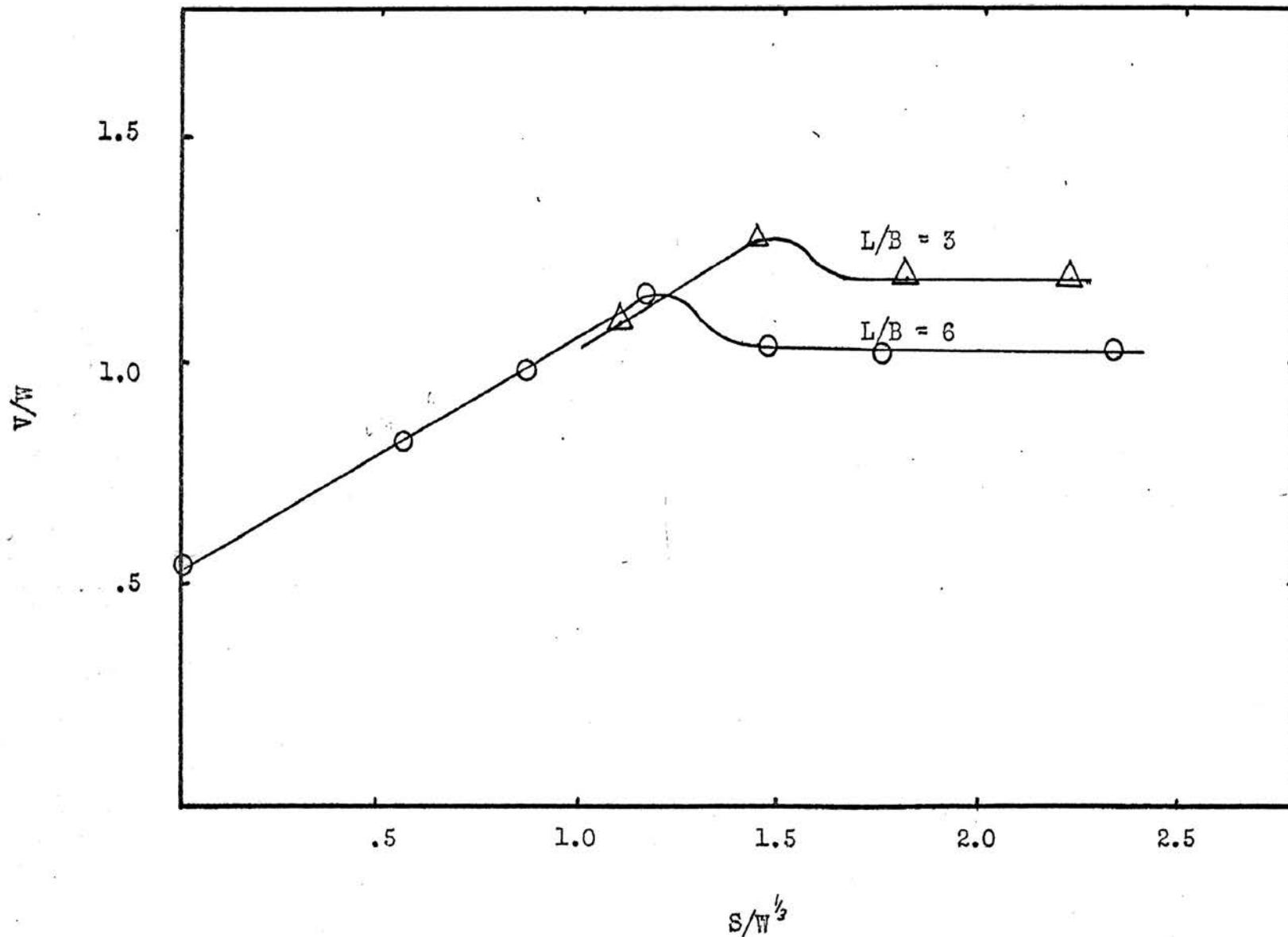
Figure 17. Crater Volume/Charge Weight vs. Explosive Spacing/(Charge Weight)<sup>1/3</sup> for Mortar (1/2 in. B)
