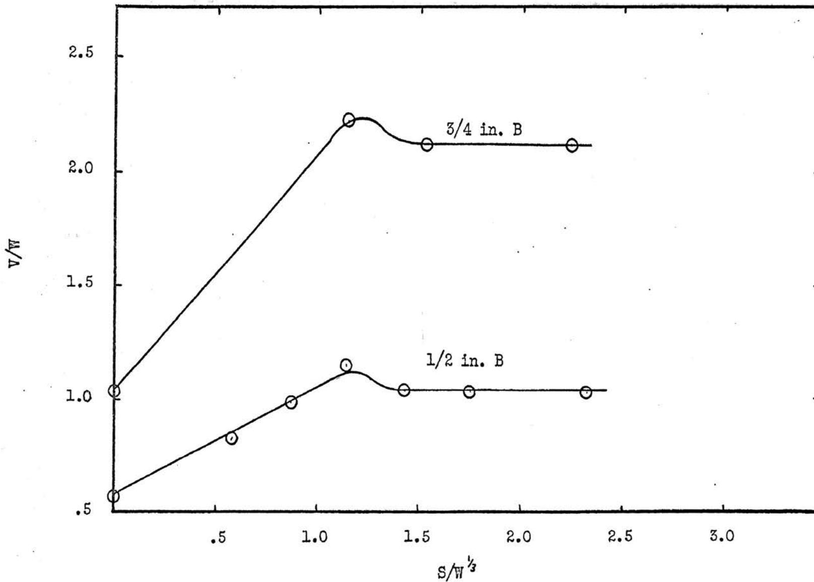
Figure 16. Crater Volume/Charge Weight vs. Explosive Spacing/(Charge Weight)<sup>1/3</sup> for Mortar (L/B = 6)
