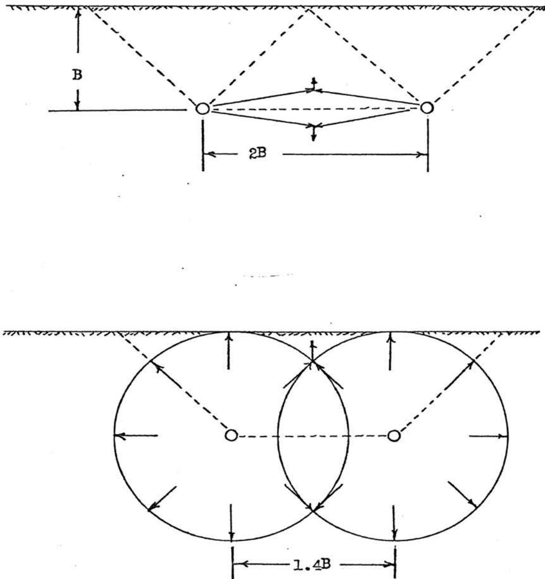
Figure 6. Spacing Relationships Determined by Geometrically Balancing Stresses in the Plane of the Charge Diameter.
