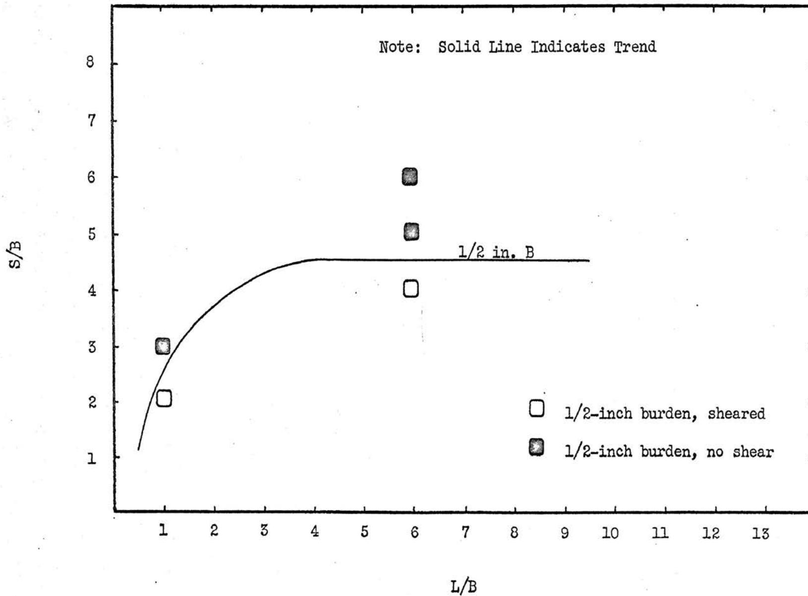
Figure 14. Explosive Spacing/Burden vs. Charge Length/Burden for Dolomite
