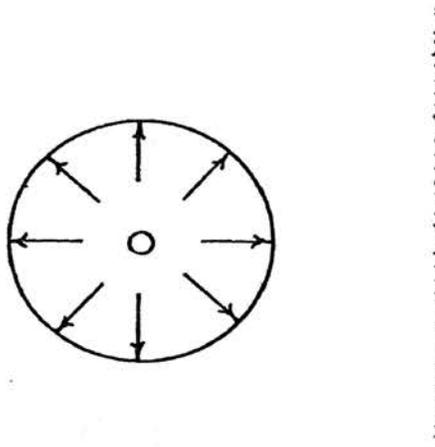
Figure 4. Conical Compressive Wave Form, Moving Down a Long Column of Detonating Explosive
