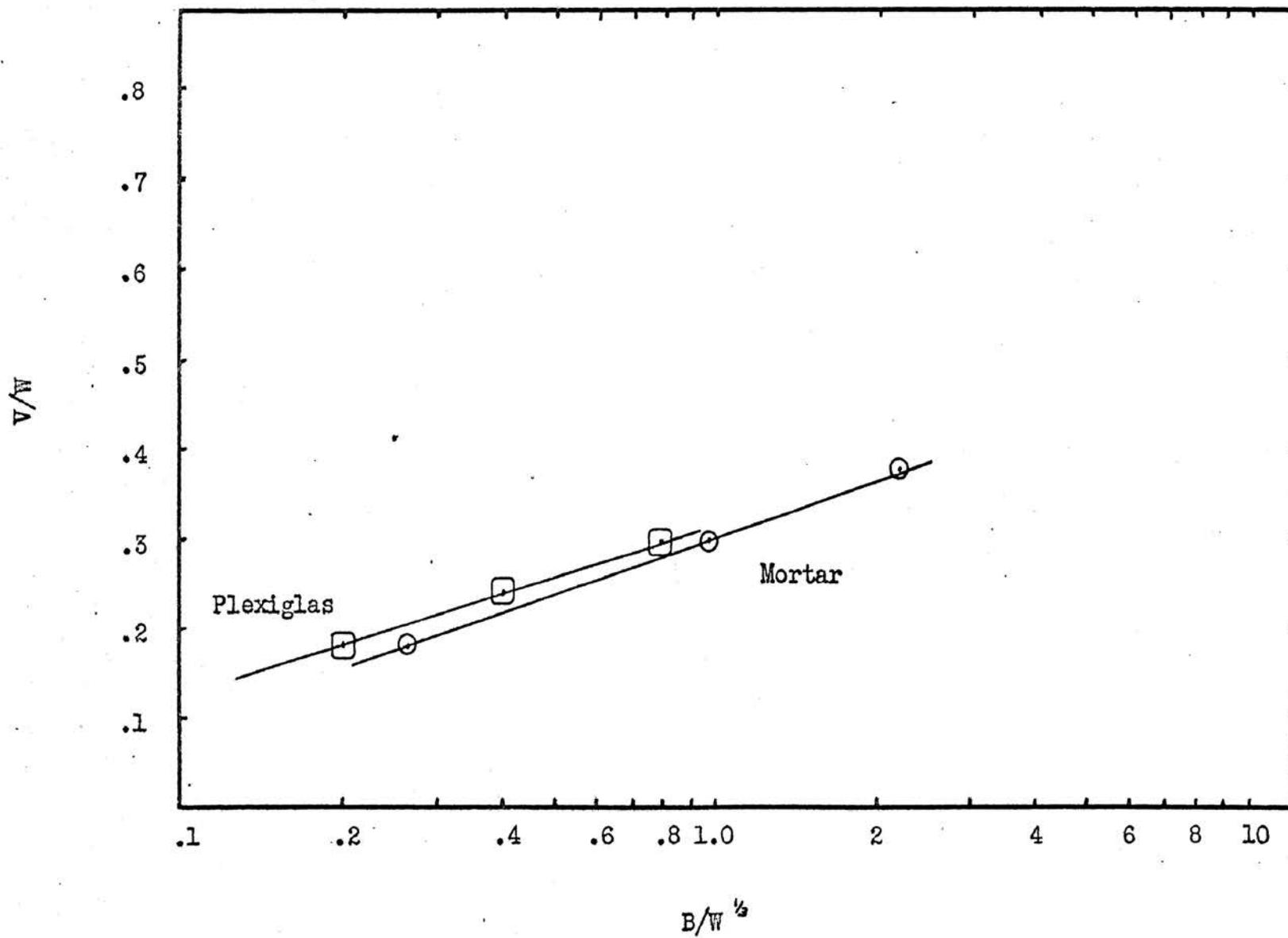
Figure 19. Crater Volume/Charge Weight vs. Burden/(Charge Weight)<sup>1/3</sup> (L/B = 6, S/B = 3).
