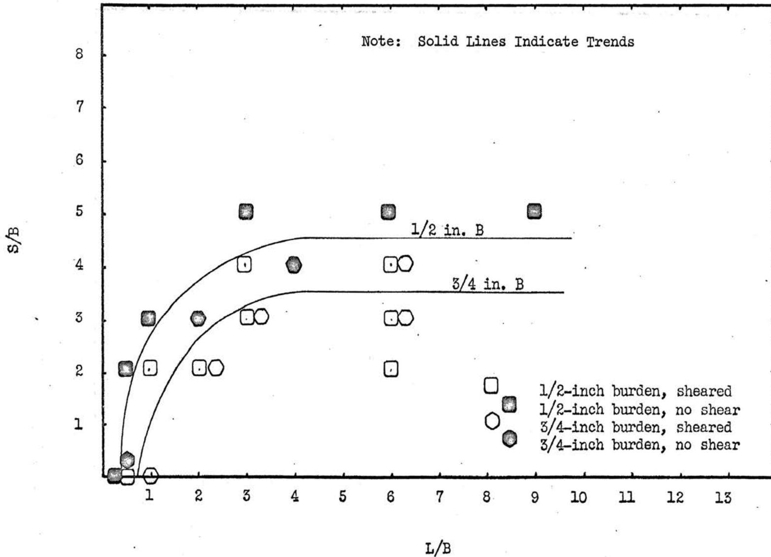
Figure 13. Explosive Spacing/Burden vs. Charge Length/Burden for Mortar
