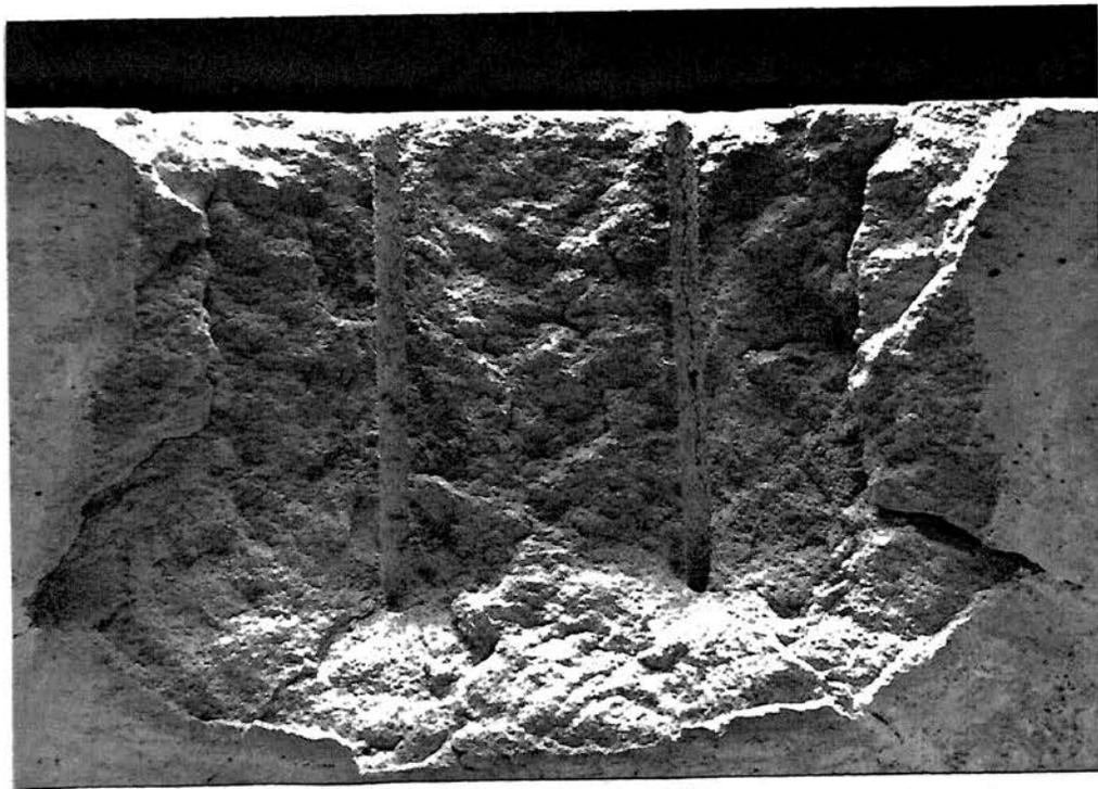
Plate VIII. MDF (10-grain) detonated in Mortar. (.75-inch Burden, Charge Length 4.5-inches, 2.25 inch spacing)
