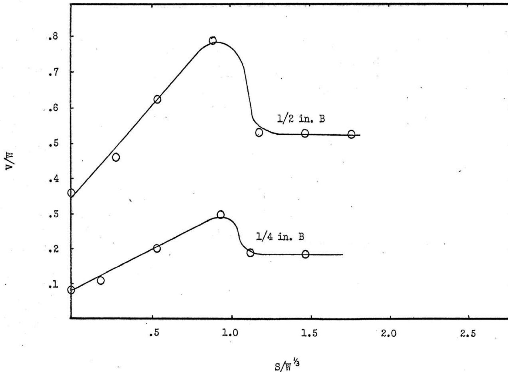
Figure 15. Crater Volume/Charge Weight vs. Explosive Spacing/(Charge Weight)<sup>1/3</sup> for Plexiglas (L/B = 6)
