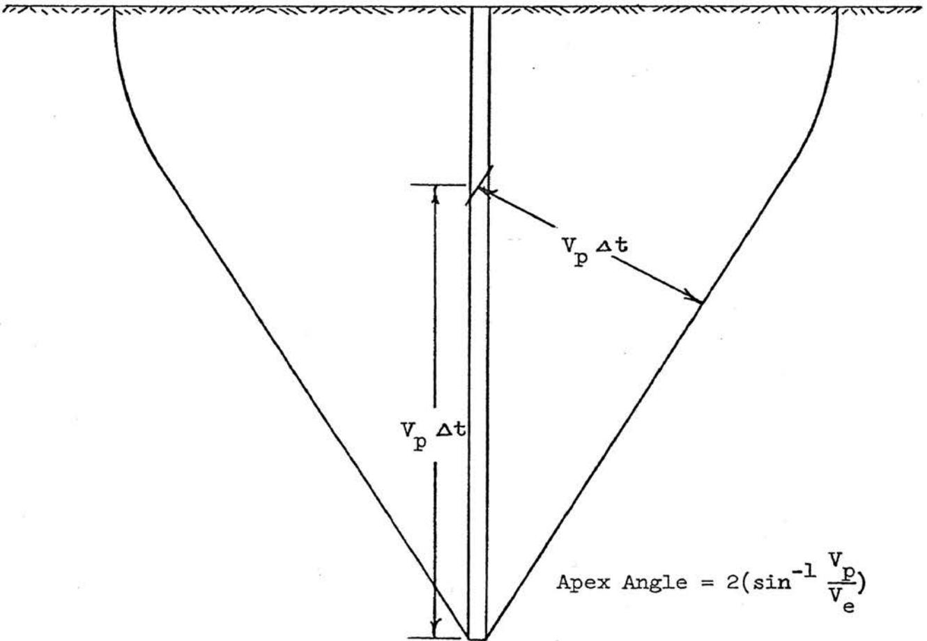
Figure 5. Angle of Conical Wave
