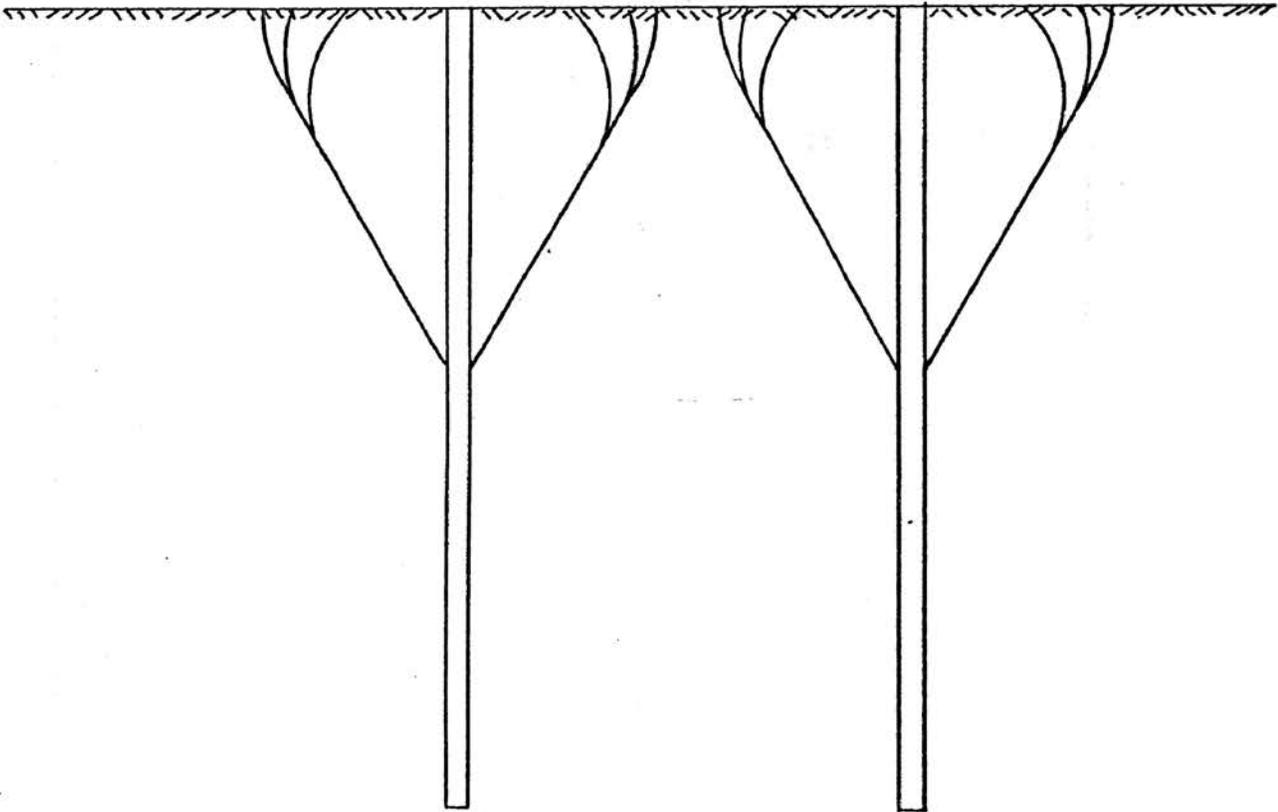
Figure 11. Noncoherent Wave Fronts between Two Simultaneously Initiated Charges
