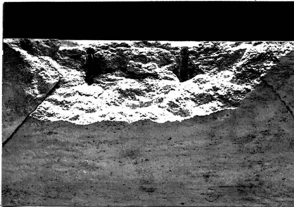
Plate X. MDF (10-grain) detonated in Mortar. (.75-inch Burden, Charge Length 1.5-inches, 2.25-inch spacing)
