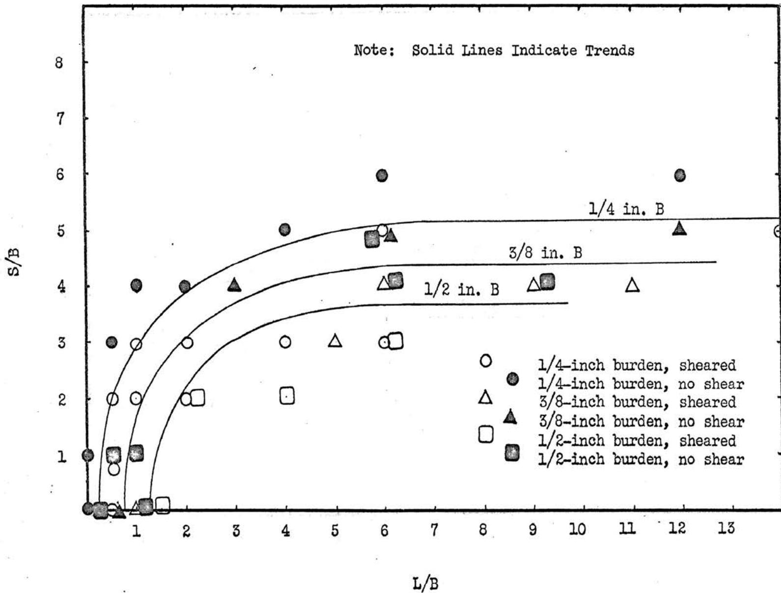
Figure 12. Explosive Spacing/Burden vs. Charge Length/Burden for Plexiglas
