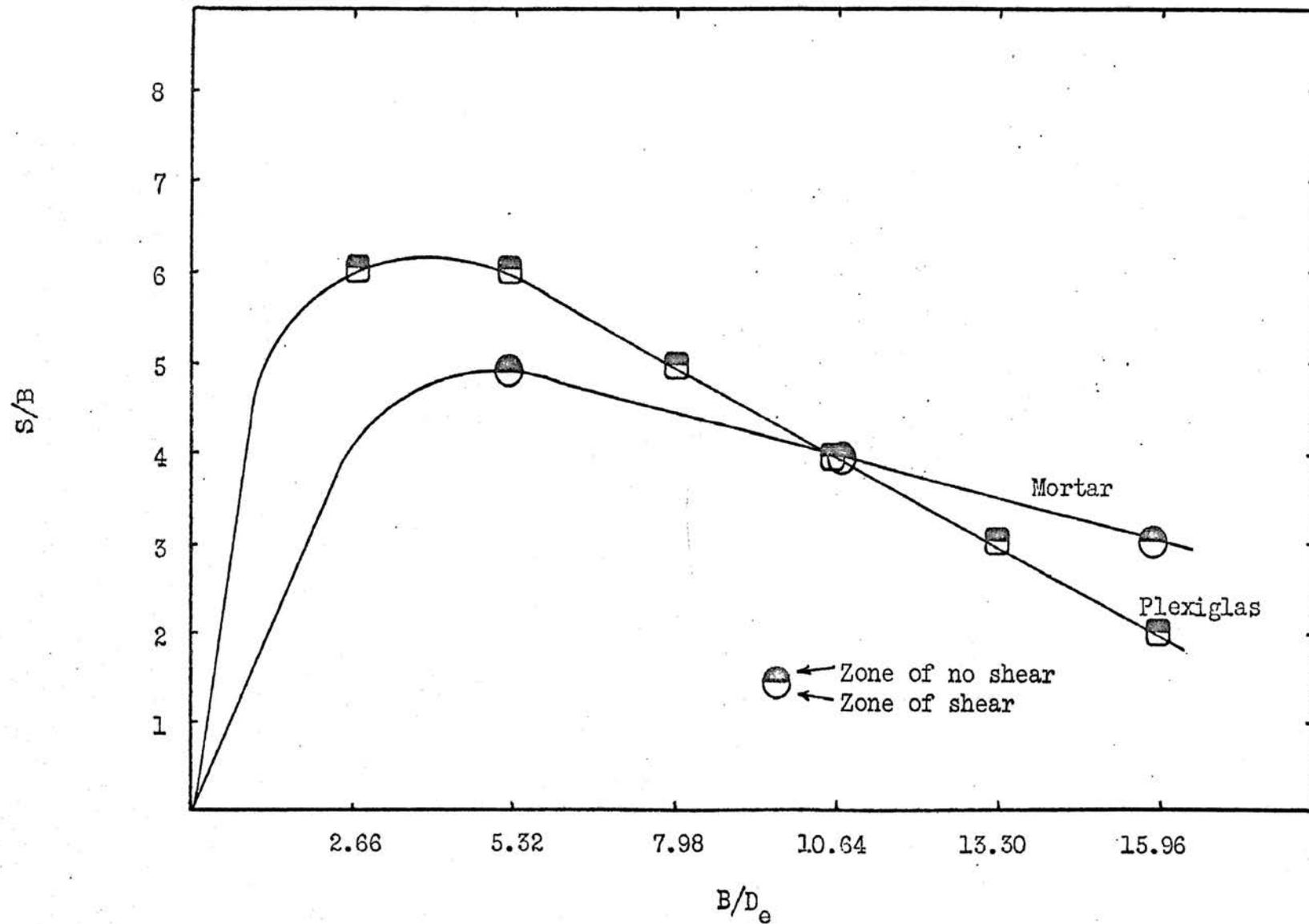
Figure 20. Charge Spacing/Burden vs. Burden/Charge Diameter (L/B = 6)
