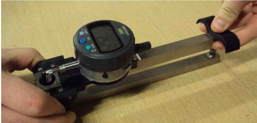
Figure 3.5 - Reading Taken on Reference Bar
