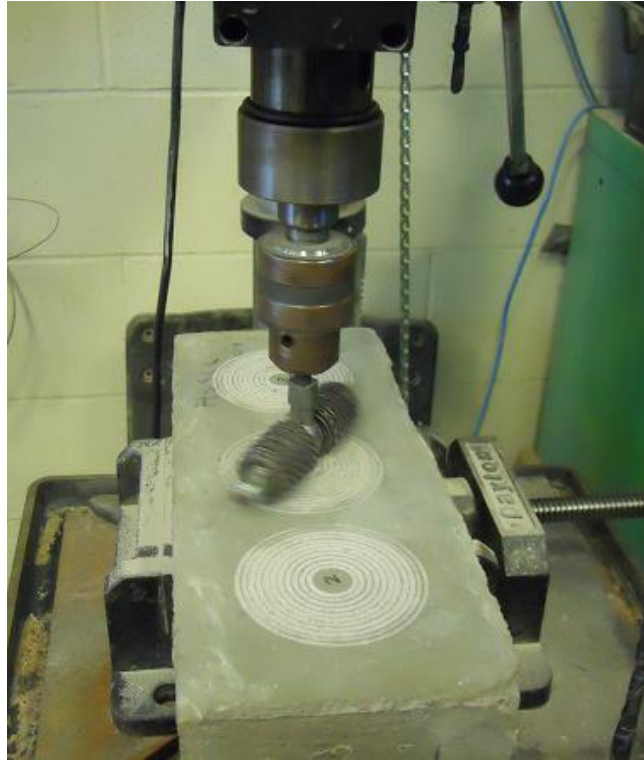
Figure 3.13 - Abrasion Resistance Test In Progress
