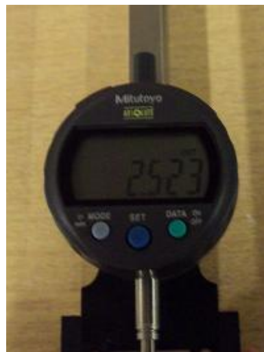
Figure 3.7 - Example DEMEC Gauge Reading
