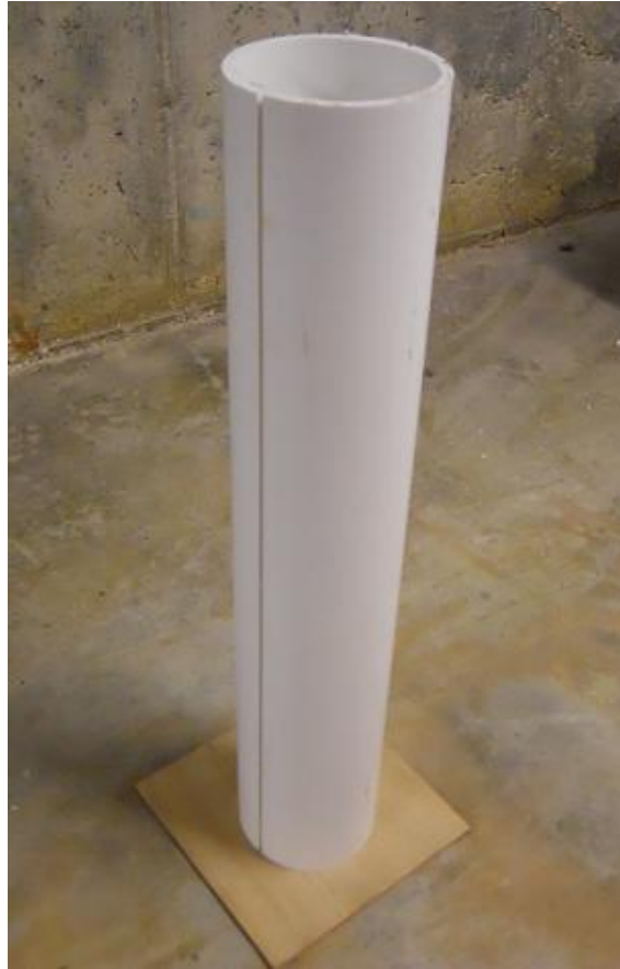
Figure 3.1 - Shrinkage and Creep Form
