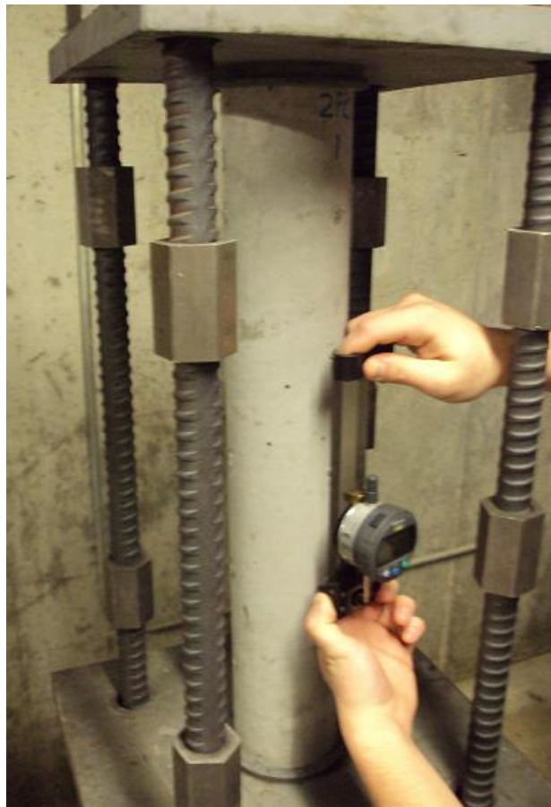
Figure 3.10 - Reading Taken on Creep Specimen
