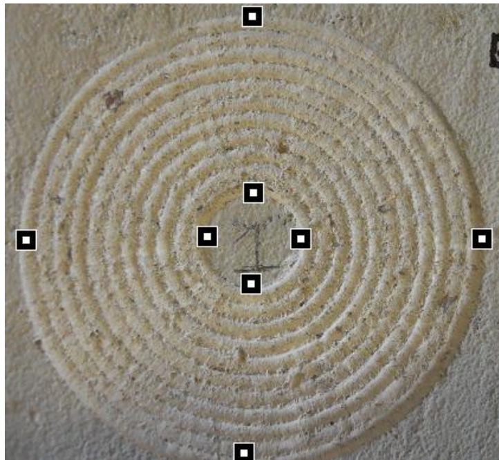
Figure 3.14 - Depth of Wear Measurement Points
