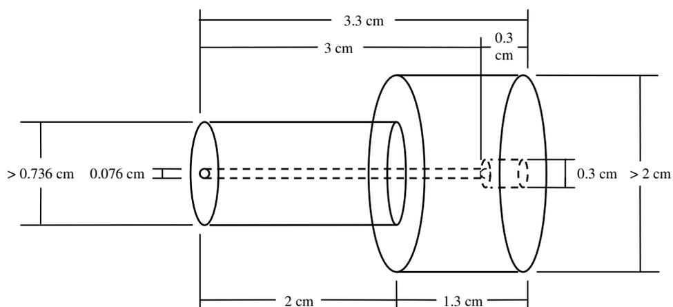
Figure 3.1. Preliminary design of SPME *in-planta* sampler.
