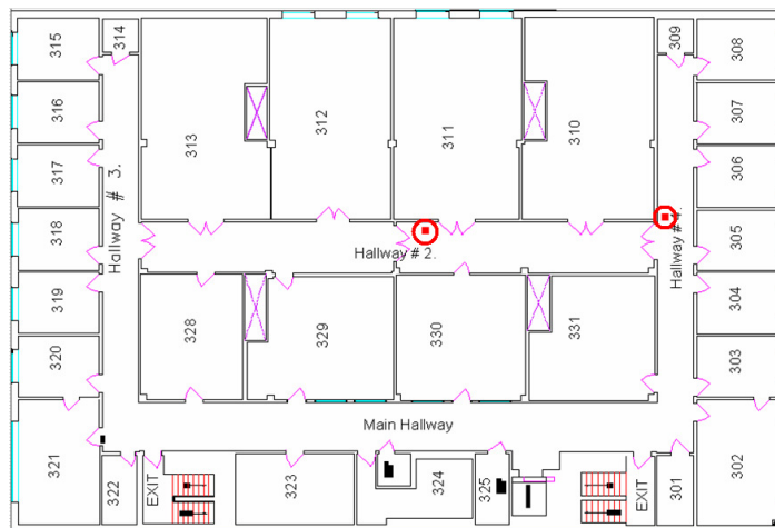
Fig. 11. Floor plan of ERL third floor. Receiver pair positions are marked with circled squares
