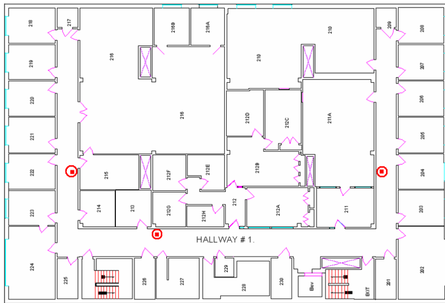
Fig. 5. Floor plan of ERL second floor. Receiver pair positions are marked with circled squares
