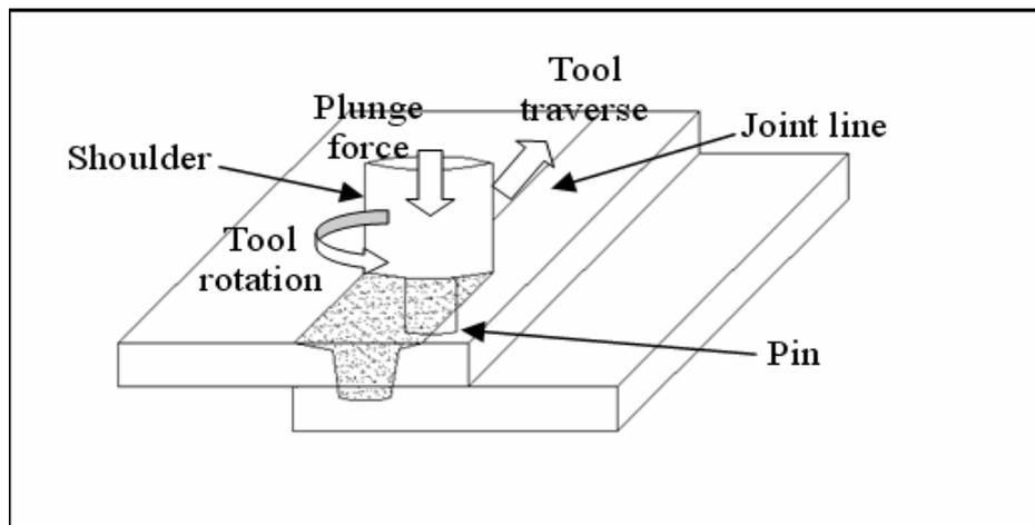
**Figure 1: Lap Weld Using FSW Process**
