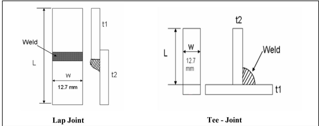
Figure 17: Test Coupons for MIG Welded Joint
