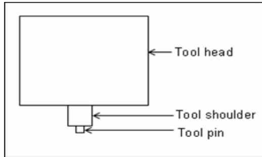
**Figure 2: FSW Tool Head and FSW Tool**
