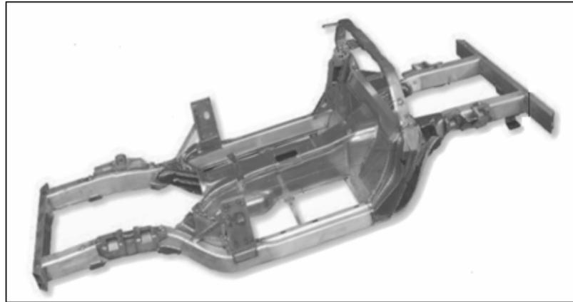
**Figure 15: Aluminum Chassis Used for Functional Feasibility Study**
