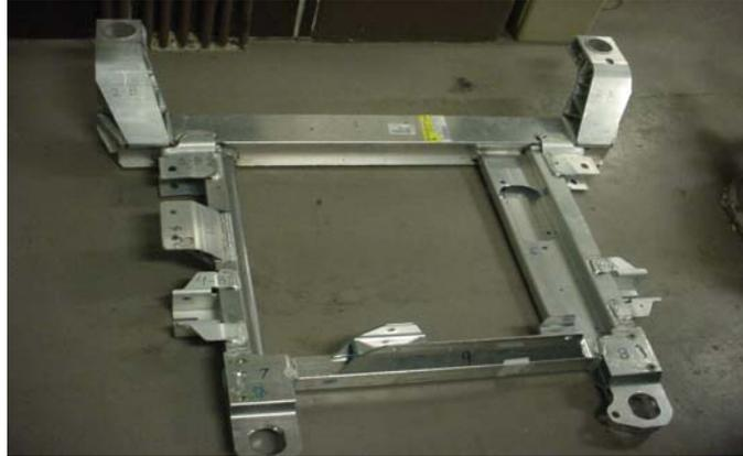
**Figure 16: Aluminum Chassis Used for Performance Feasibility Study**
