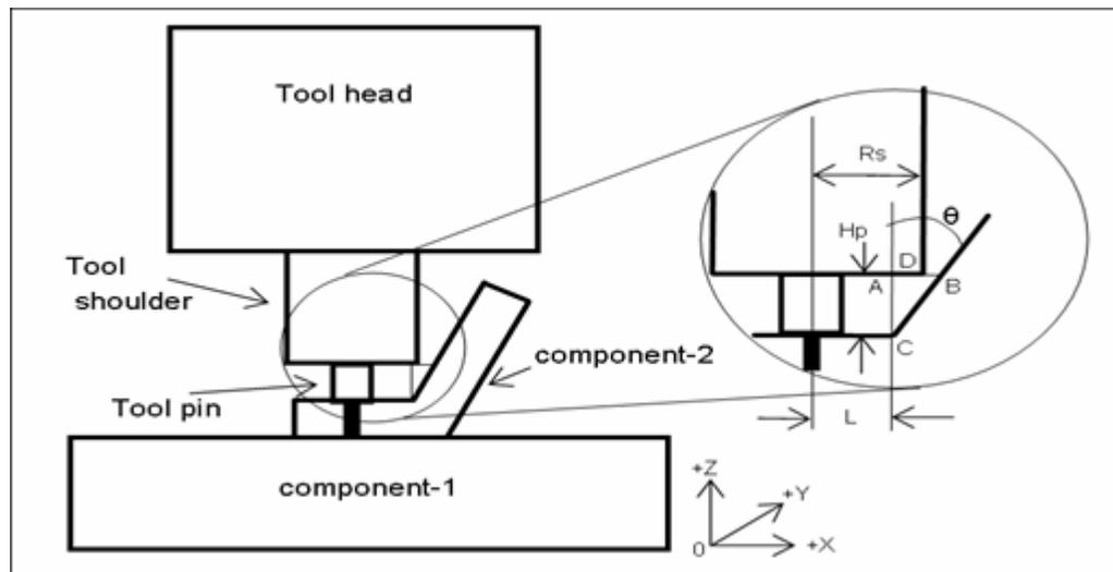
**Figure 4: Avoidance of Tool Shoulder Interference With Component-2**
