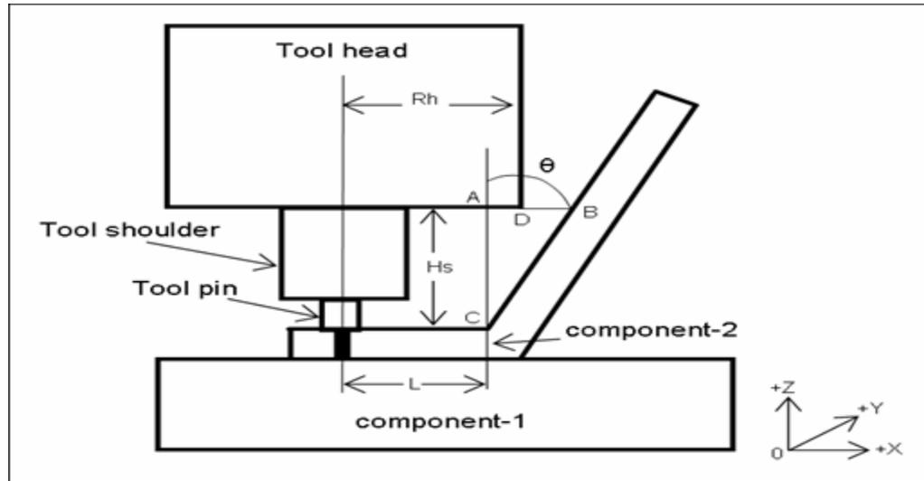
**Figure 5: Avoidance of Tool Head Interference With Component-2**
