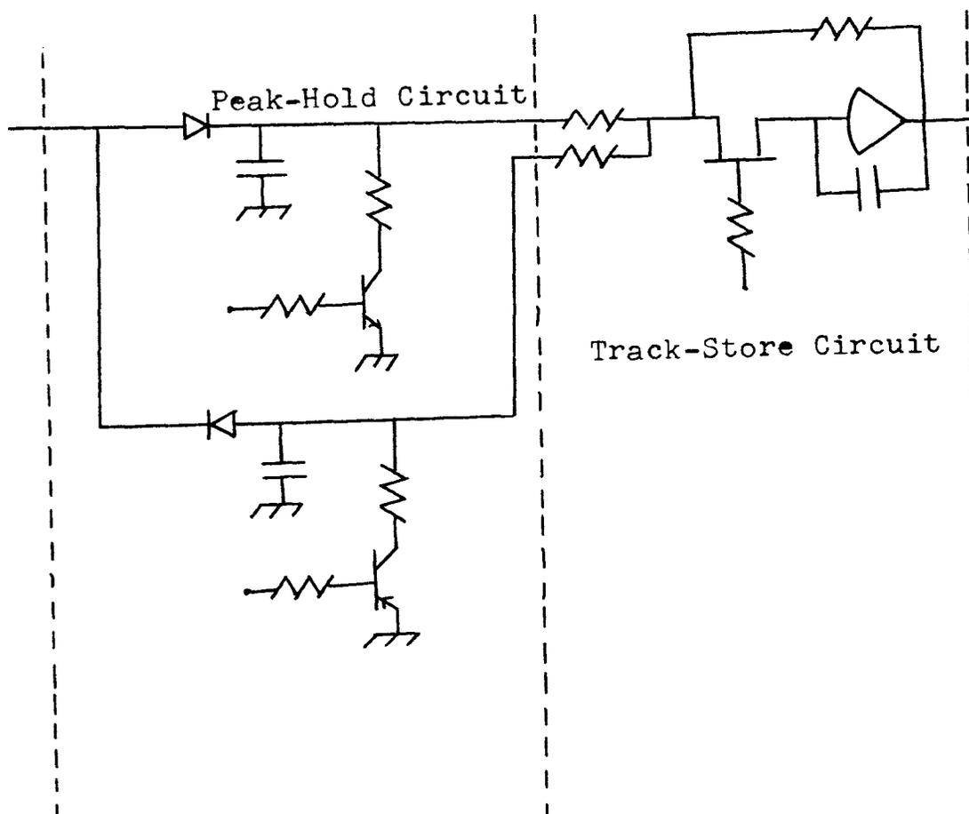
Figure 14. Peak-Hold Circuit
