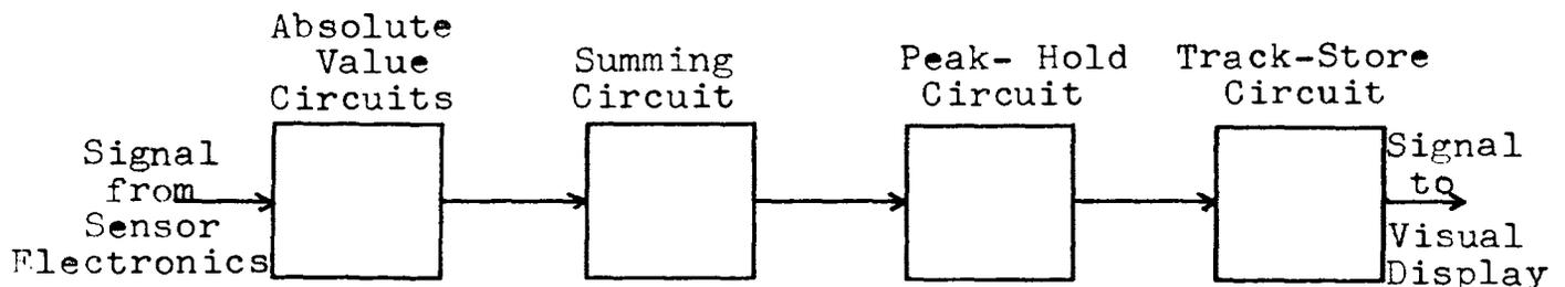
Figure 3. Block Diagram of Signal Processing
