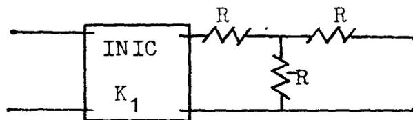
Figure 5. Gyrator Realization Using NIC
