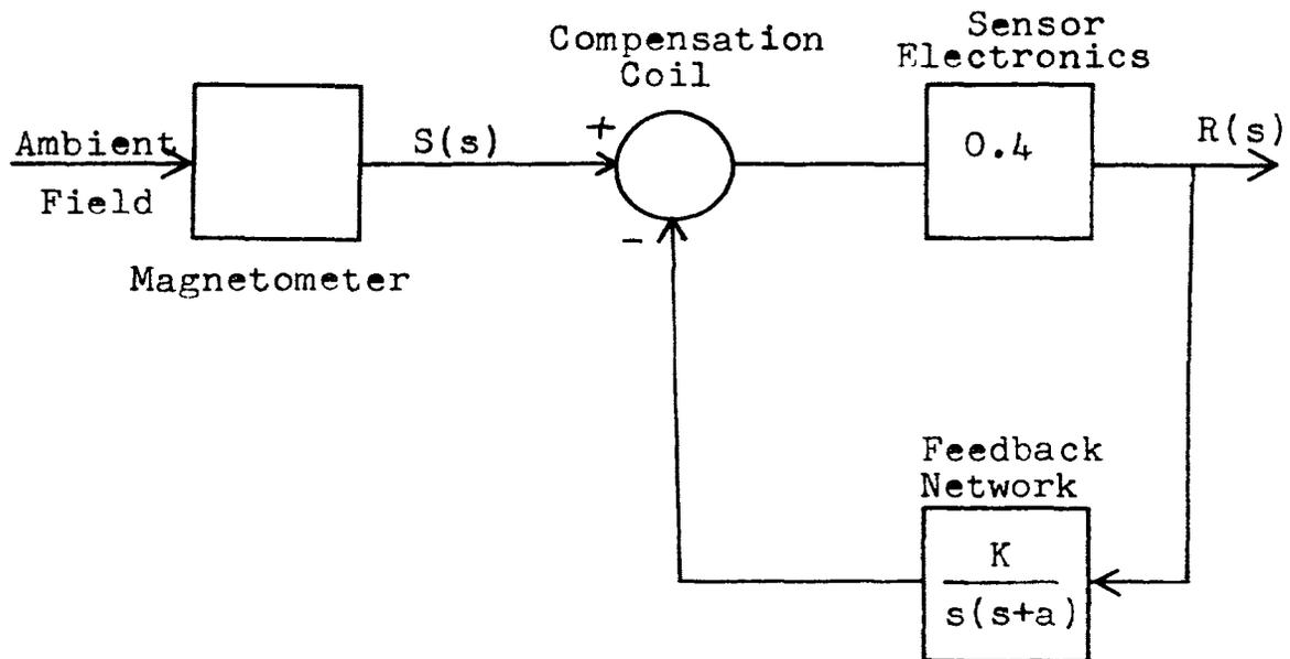
Figure 4. Block Diagram Involving Feedback Network
