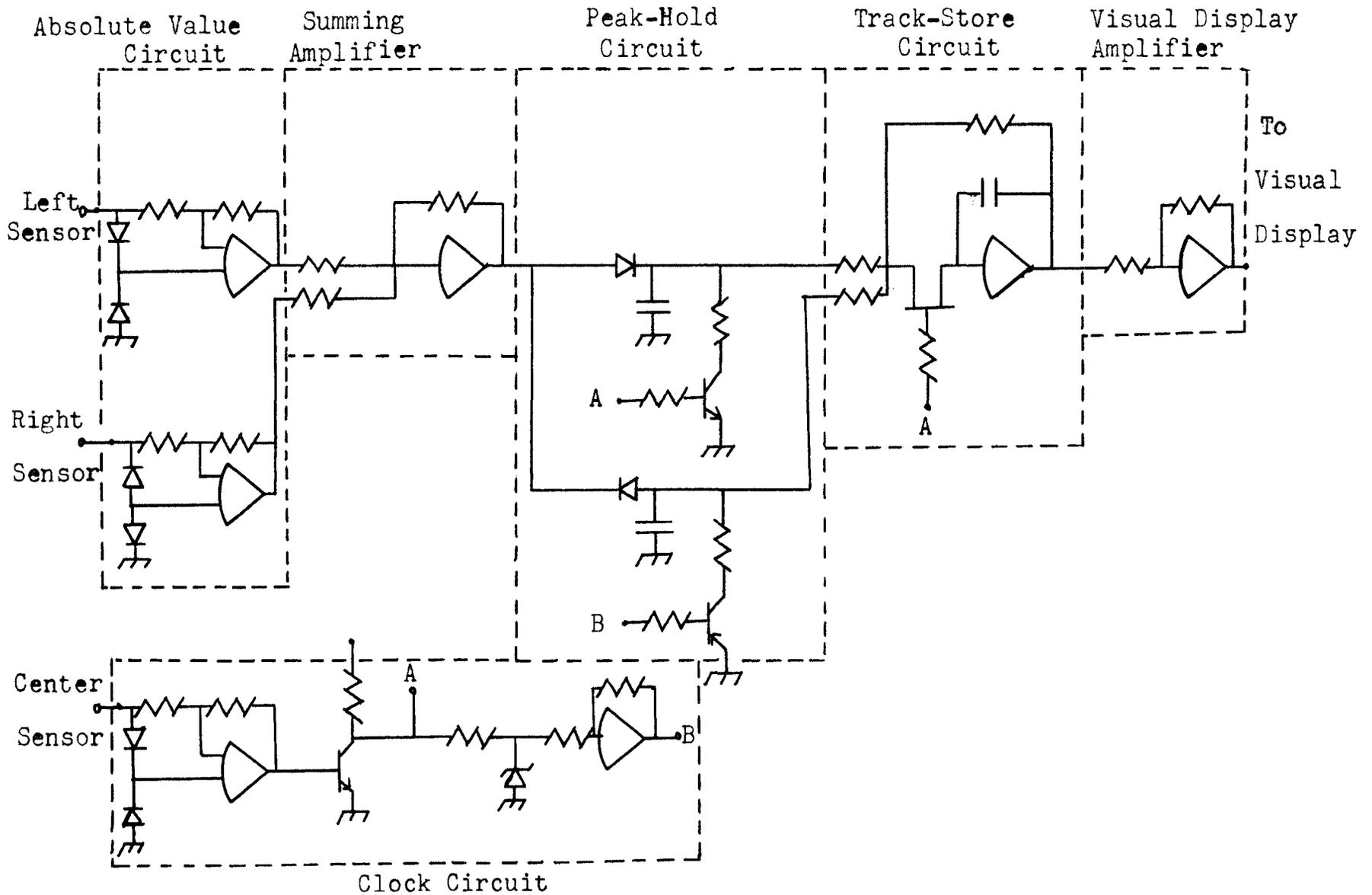
Figure 13. Signal Processing Electronics
