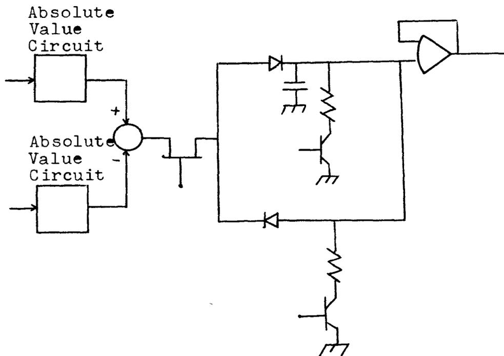
Figure 15. Proposed Signal Processing
