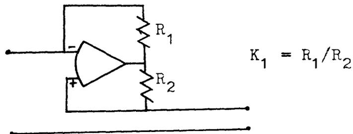
Two operational amplifiers are required to realize Figure 4; one operational amplifier to construct the INIC, another to realize the  $-R$  element.
