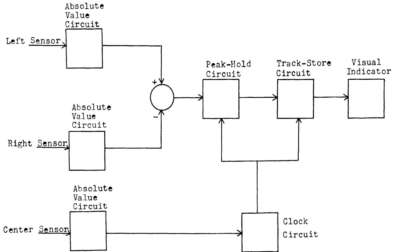
Figure 9. Block Diagram of Signal Processing
