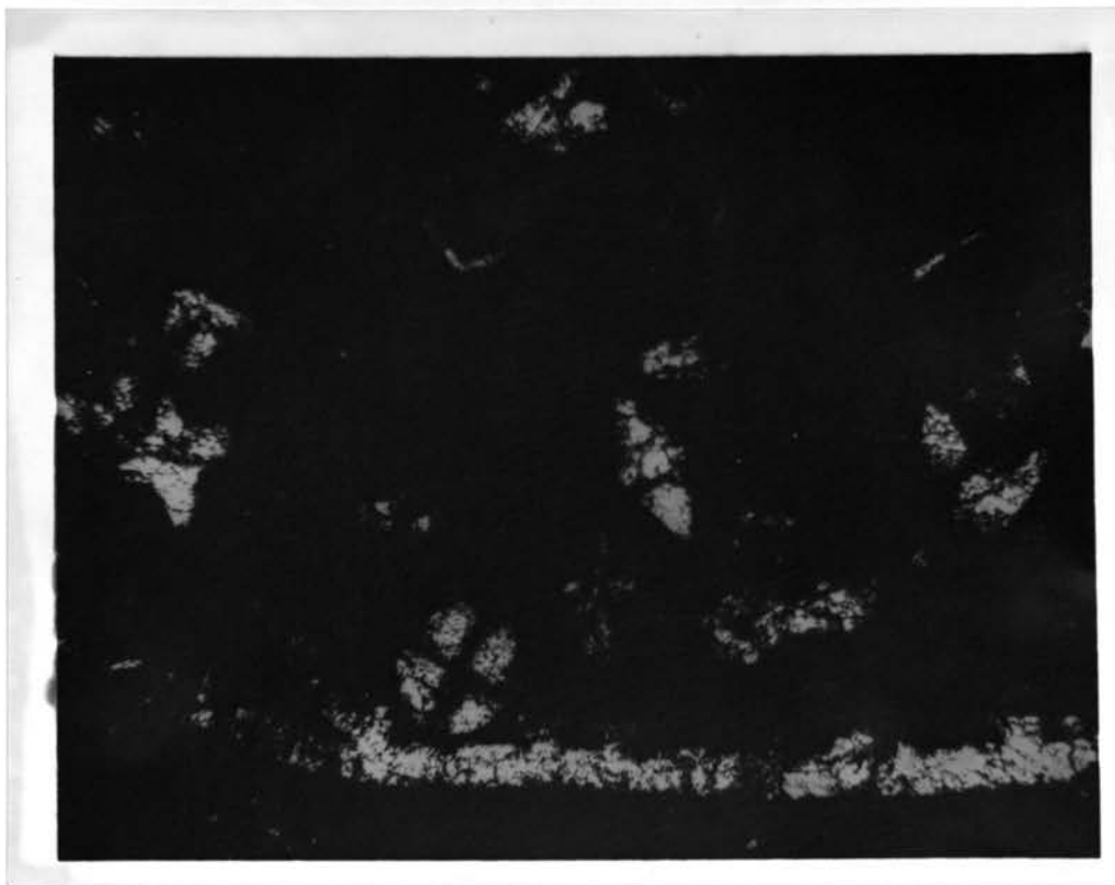
Figure 19. Photomicrograph of a glass-ceramic specimen heat-treated according to point 1.0 (Figure 14) viewed with transmitted light under crossed nicols. 16X
