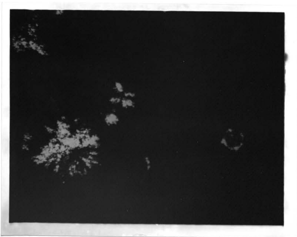
Figure 22. Photomicrograph of a glass-ceramic specimen heat-treated according to point 1.1 (Figure 14) viewed with transmitted light under crossed nicols. 20X
