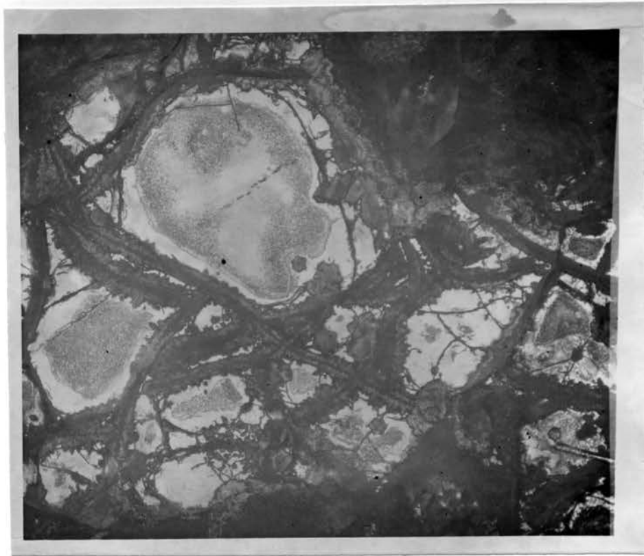
Figure 36. Photomicrograph of a glass-ceramic specimen heat-treated according to point 2.1 (Figure 14) viewed with reflected light under uncrossed nicols. 60X
