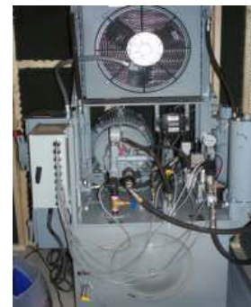
Fig. 14. Picture of the axial piston pump testbed.
