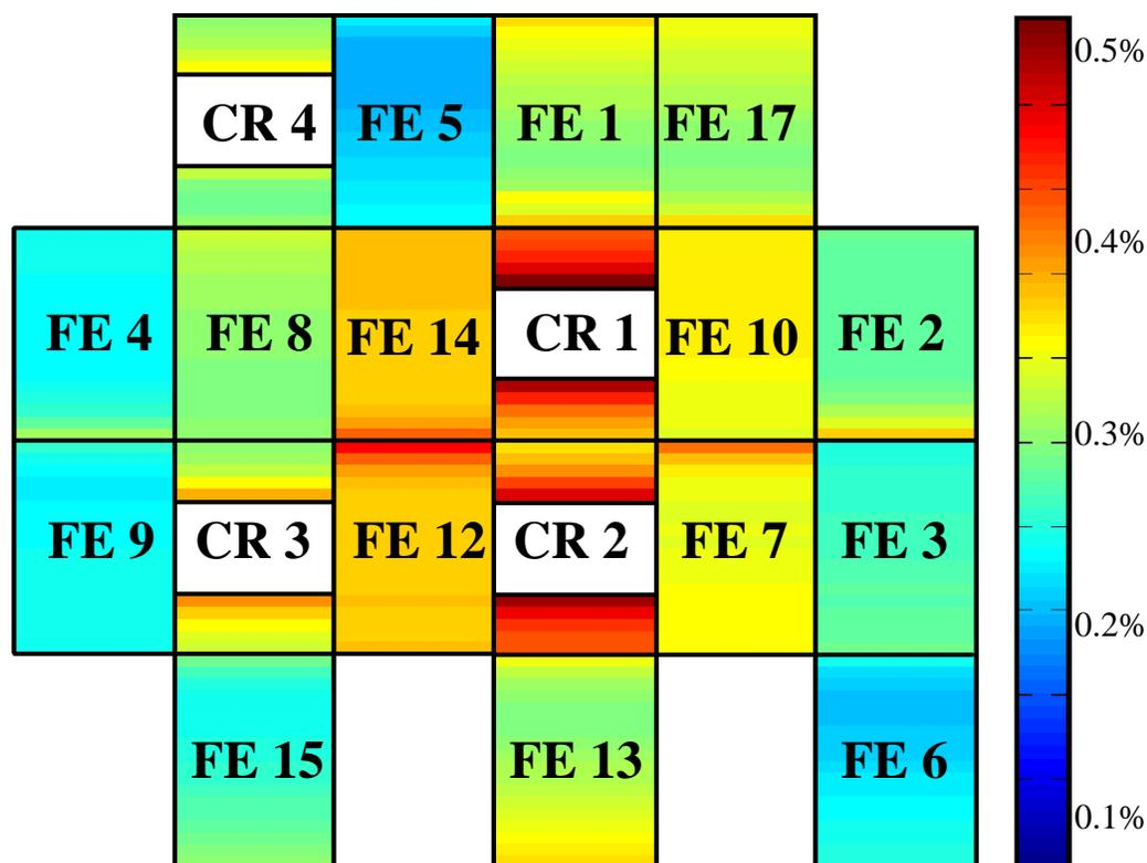
Figure 4.7. Fractional energy deposition in plates with updated fuel material
