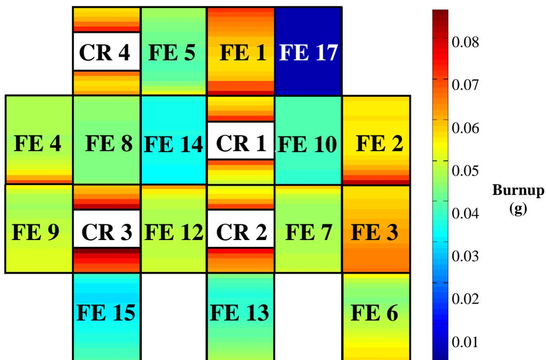
Figure 3.4.  $^{235}\text{U}$  fuel plate burnup map, Core Configuration 120
