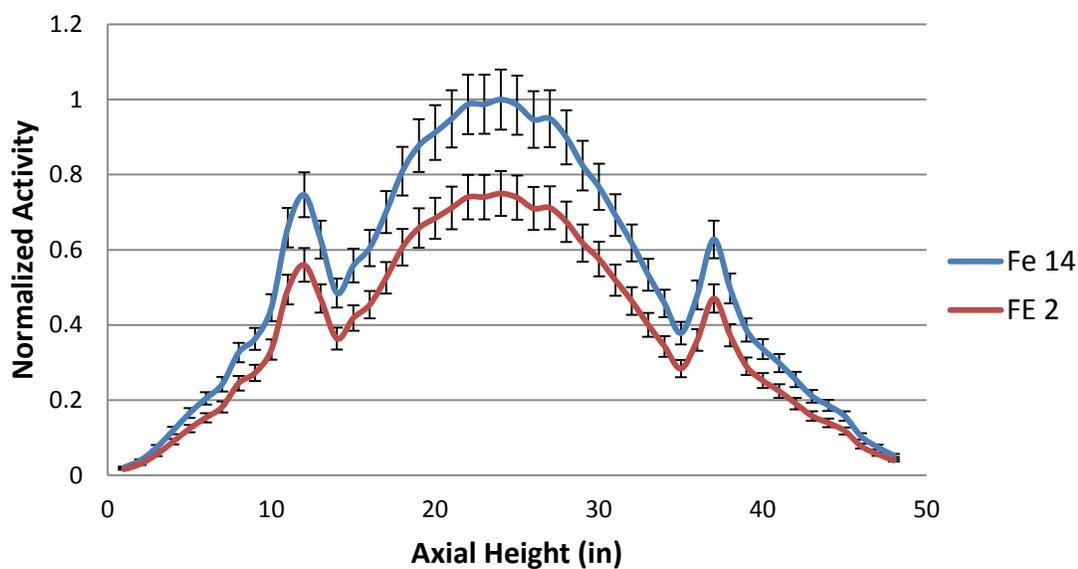
Figure 4.5. Experimentally measured axial flux profile, fuel elements fourteen and two
