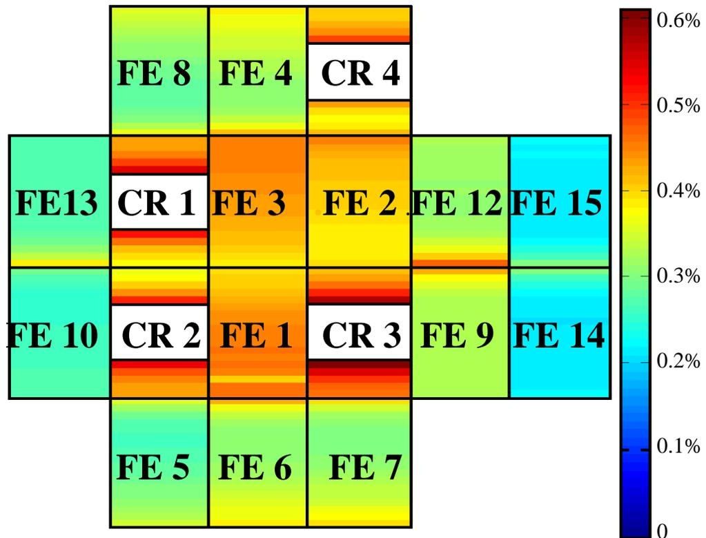
Figure 2.2. Fractional energy deposition in fuel plates, Core Configuration 101
