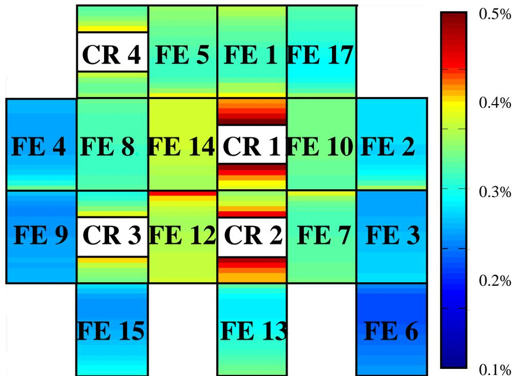
Figure 2.3. Fractional energy deposition fuel plates, Core Configuration 120
