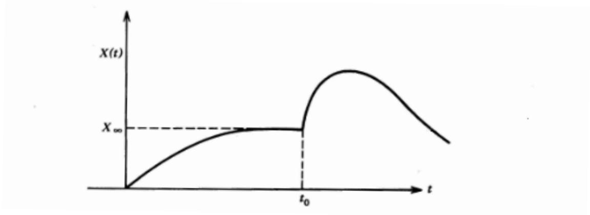
Figure 3.2. Qualitative behavior of  $^{135}\text{Xe}$  concentrations following a cold, clean startup and then shutdown
