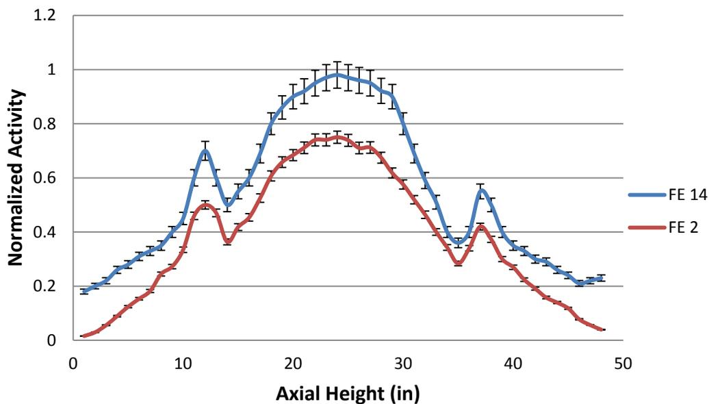
Figure 4.6. Simulated axial flux profile, fuel elements fourteen and two
