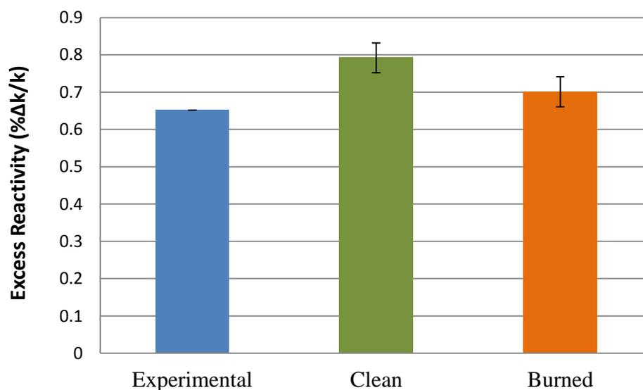
Figure 4.2. Excess reactivity comparison between experimental, clean, and burned calculations for MSTR Core Configuration 120
