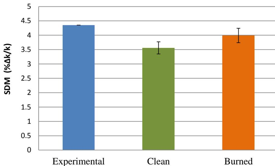
Figure 4.3. Shutdown margin comparison between experimental, clean and burned calculations for MSTR Core Configuration 120
