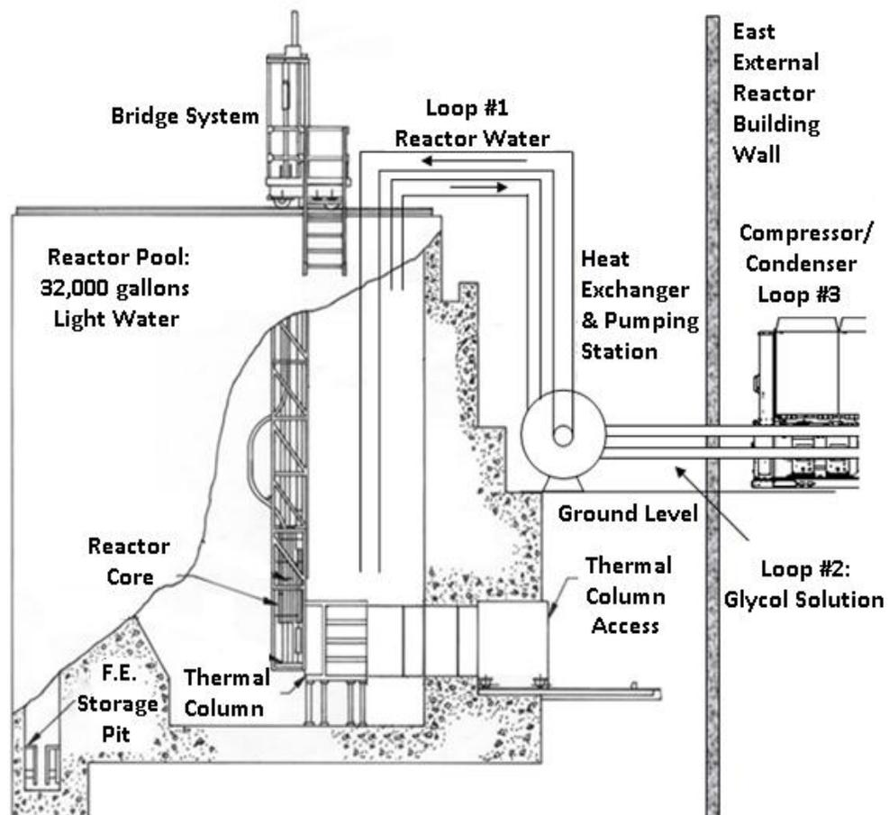
Figure 1.1. MSTR system schematic
