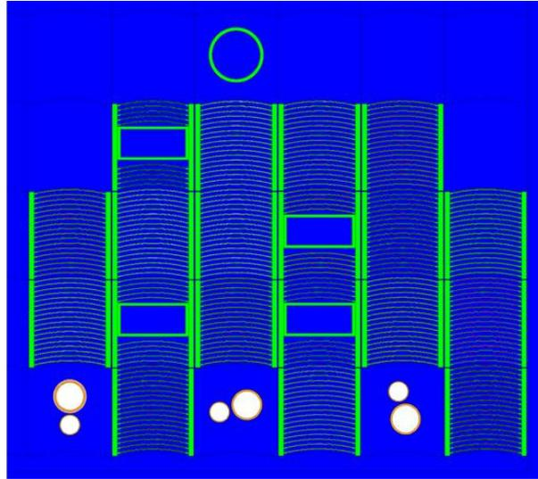
Figure 1.8. MCNP overhead view of MSTR Core Configuration 120
