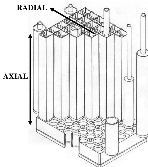
Figure 1.9. Reference directions of MSTR core
