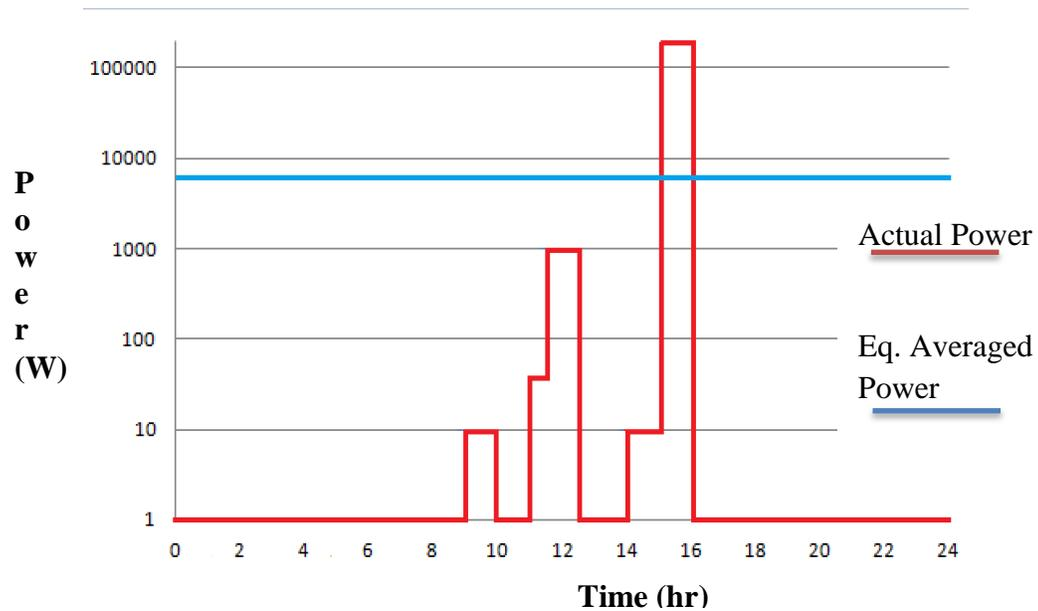
Figure 3.1. MSTR actual operational power and equivalent averaged power
