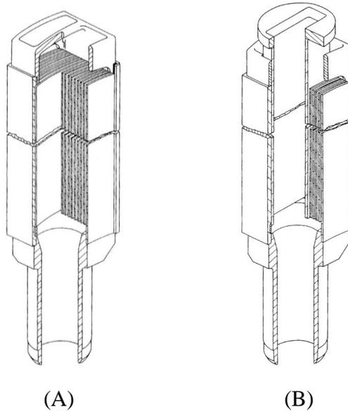
Figure 1.3. Fuel elements, (A) standard and (B) control rod
