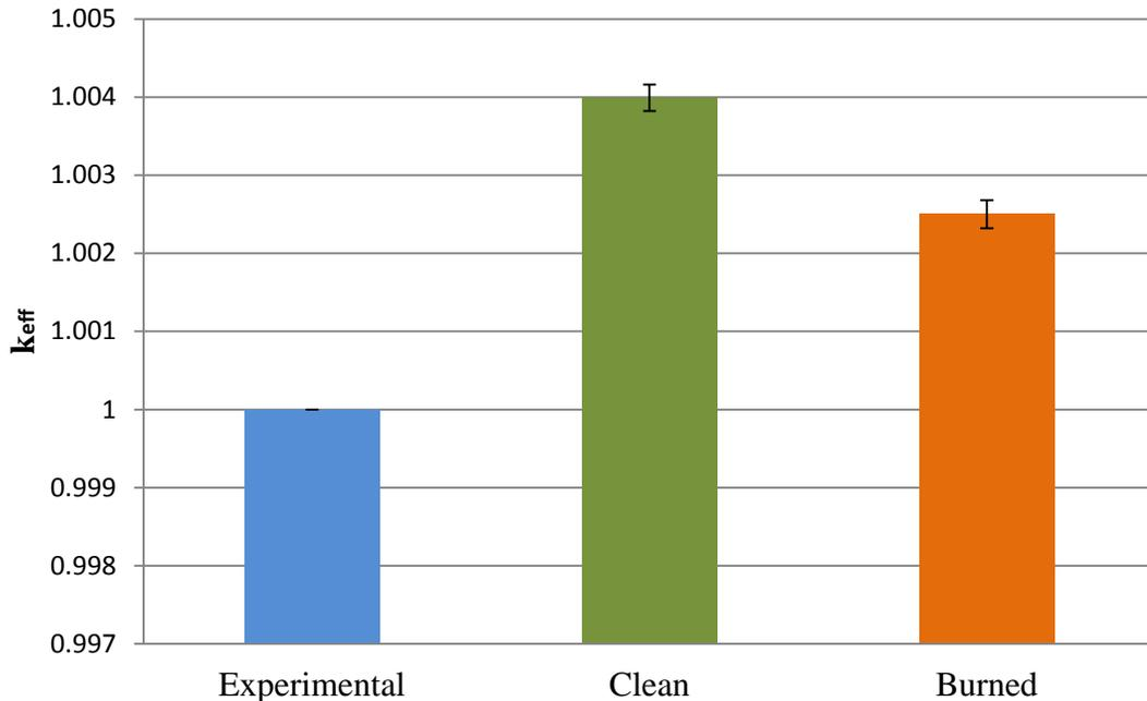
Figure 4.1. Comparison of  $k_{eff}$  values for burned and clean models at experimentally measured critical rod heights.
