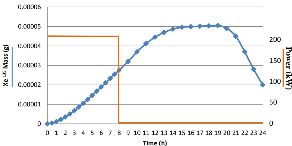
Figure 3.3.  $^{135}\text{Xe}$  buildup in MSTR during eight hour operation at 200 kW and after shutdown
