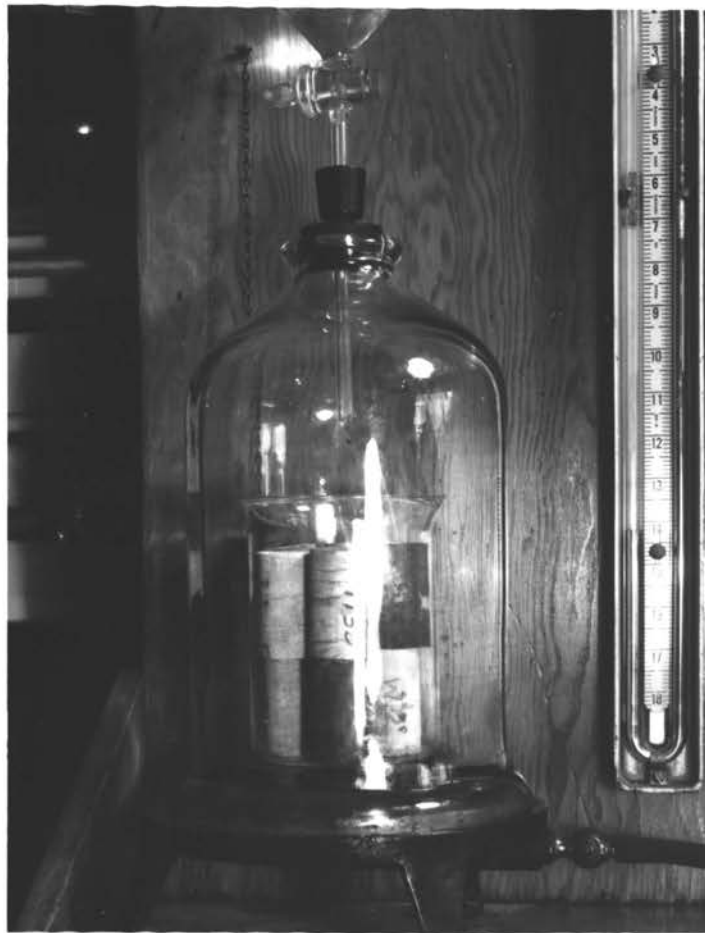
Figure 25 Water was Added Slowly to Allow for Complete Saturation of the Pore Area.
