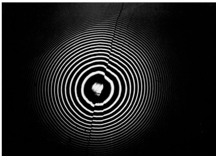
Figure 42. Zn-Mg alloy, 0.005% Mg, single crystal, basal plane. Interference pattern of unetched cleavage surface. "step" on the surface. Magnification 165X.
