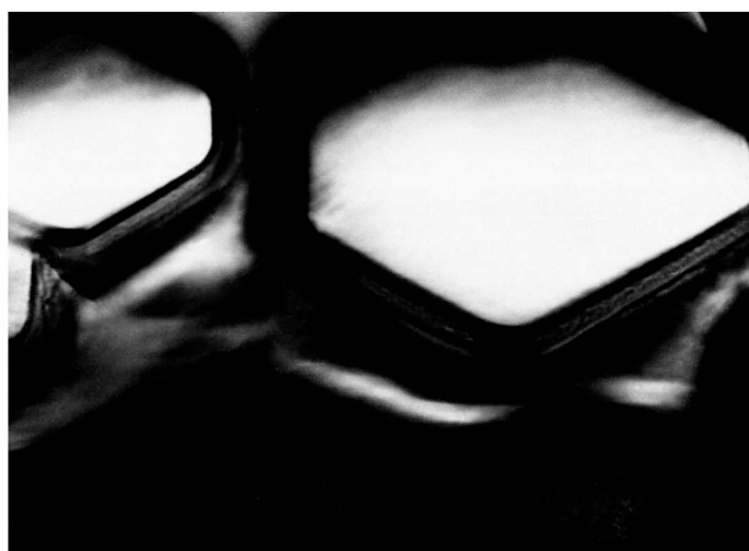
Figure 19. Zn (99.99%), single crystal, basal plane, etched in 9.5N \text{HNO}_3 for 5 sec. above - Top of etch pits. Mag. 750X. below - Bottom of etch pits. 1430X.
