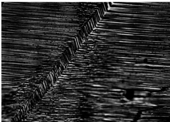
Figure 51. Zn-Mg alloy, 0.01% Mg, single crystal, prismatic plane 1st. order, etched in 12N HCl for 5 sec. Magnification 1430X.
