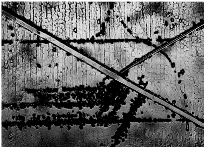
Figure 43. Zn-Mg alloy, 0.005% Mg, single crystal, basal plane, etched in 2N HCl for 20 sec. Magnification 145X.
