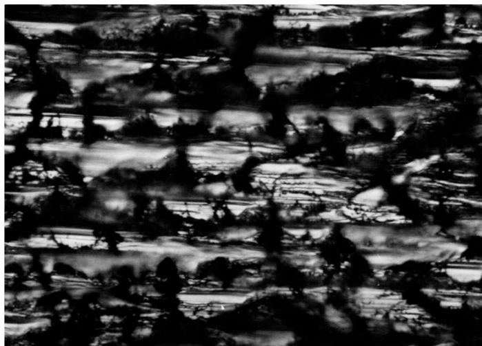
Figure 33. Zn-Au alloy, 0.04% Au, single crystal, prismatic plane 1st. order, etched in 2N HCl for 2 min. Magnification 750X.
