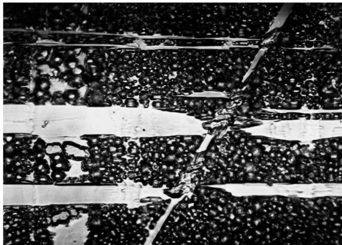
Figure 50. Zn-Mg alloy, 0.025% Mg, single crystal, basal plane, etched in 2N HCl for 1 min. Magnification 750X.
