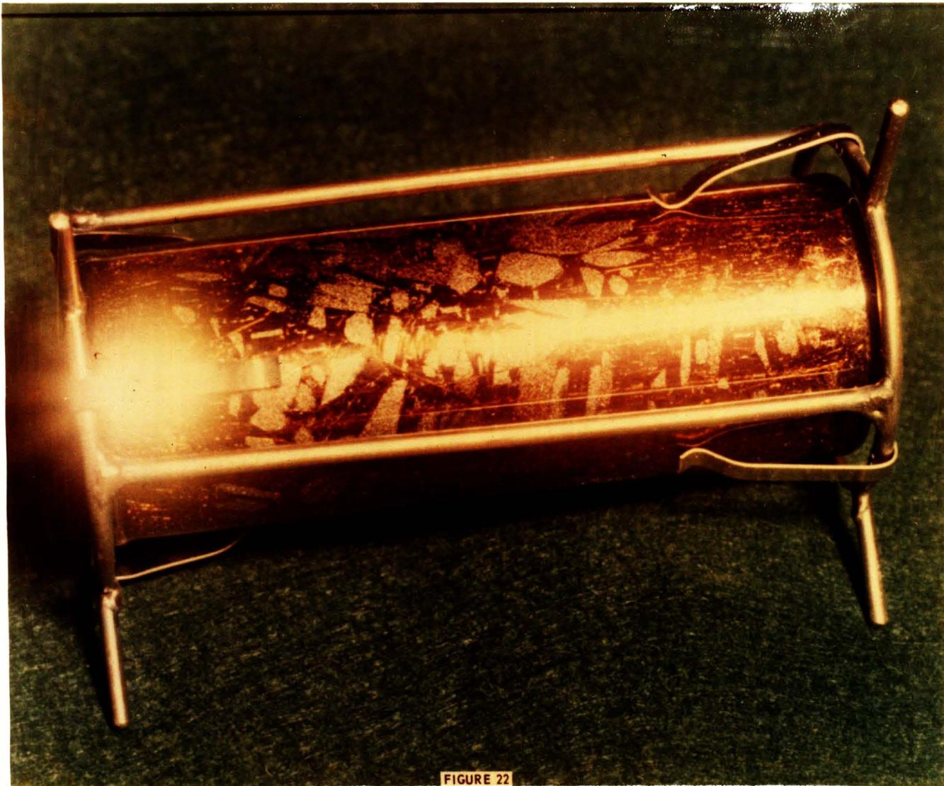
SIDE VIEW OF CORRODED PYREX CELL
