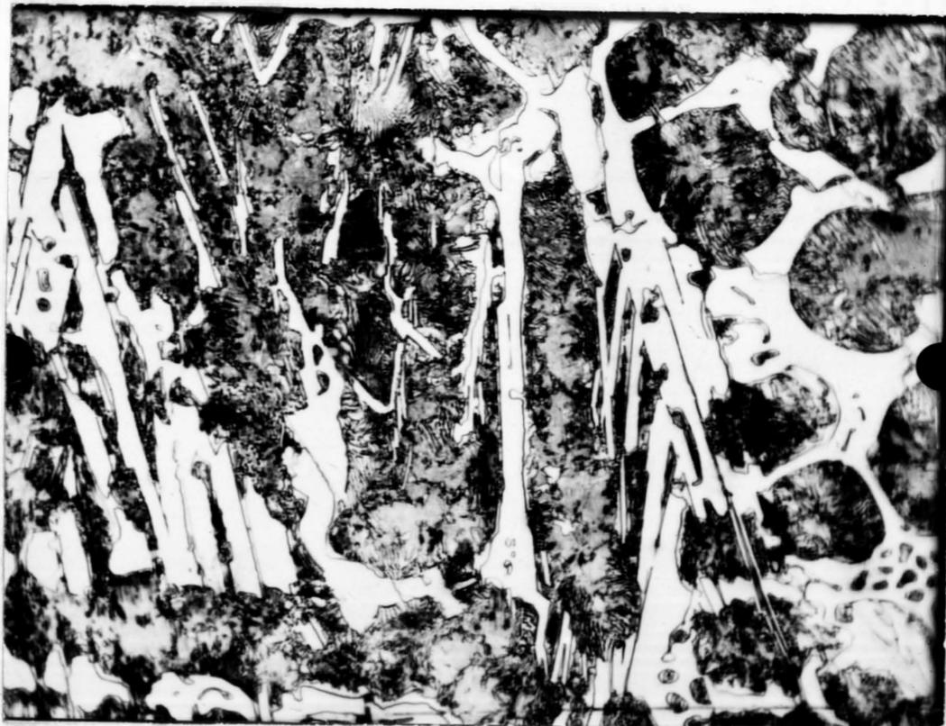
Micrograph No. 1    Sample as cast    1000 x
