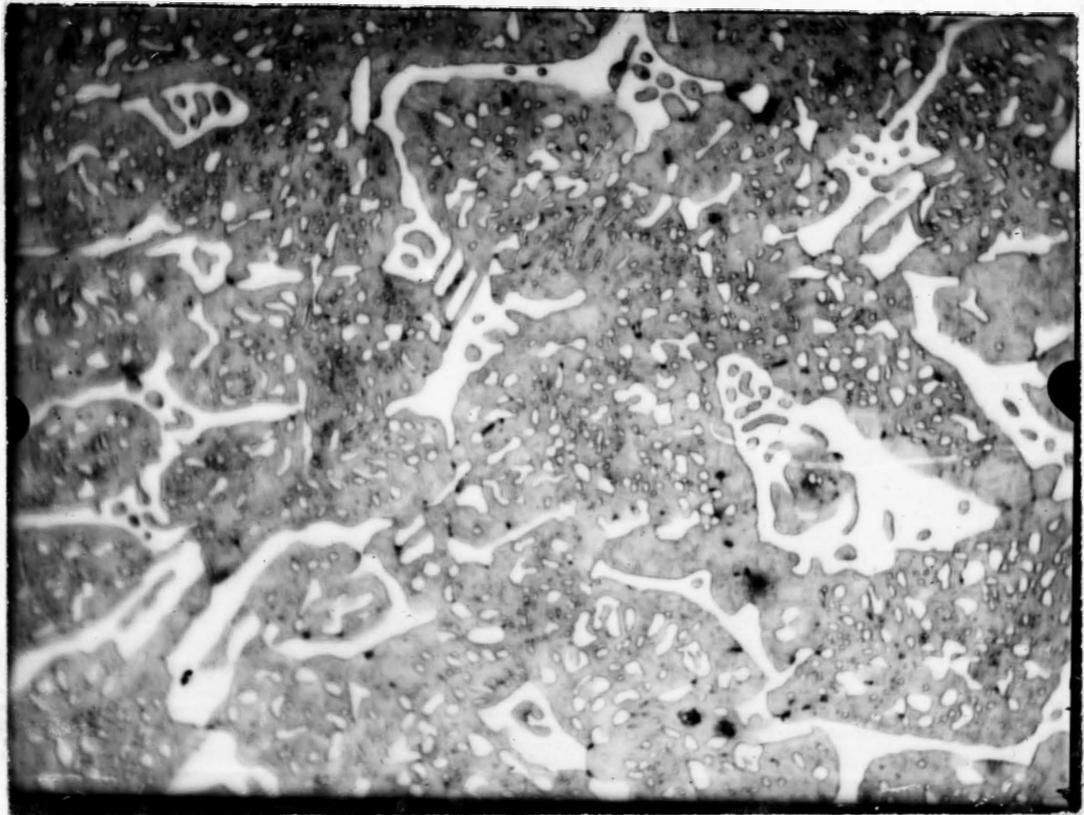
No. 6 Annealed at  $800^{\circ}$  C for 320 minutes 1000 x
