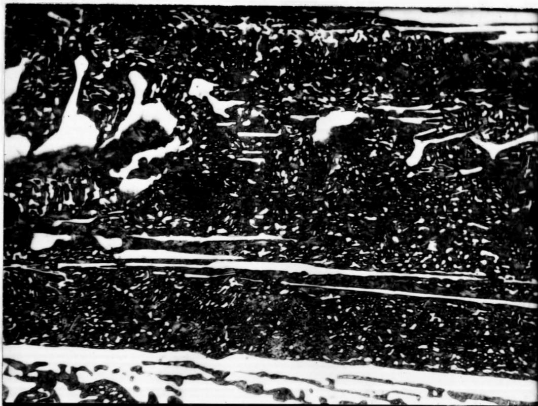
No. 2 Annealed at  $800^{\circ}$  C for 20 minutes
