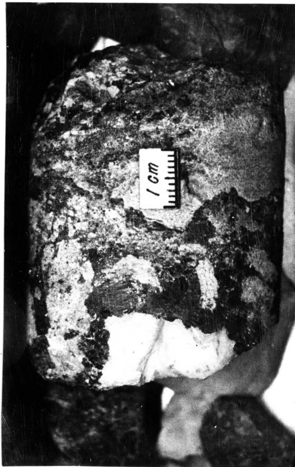
Figure 14 - Barite, sphalerite and galena as matrix in the breccia of the Krueger Zinc Deposit. Location: Hole 34,186 feet depth, U. S. Bureau of Mines Core Library, Minneapolis.
