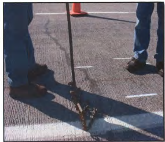
a) The automated chain drag system (ACDS). b) Manual chain dragging.
