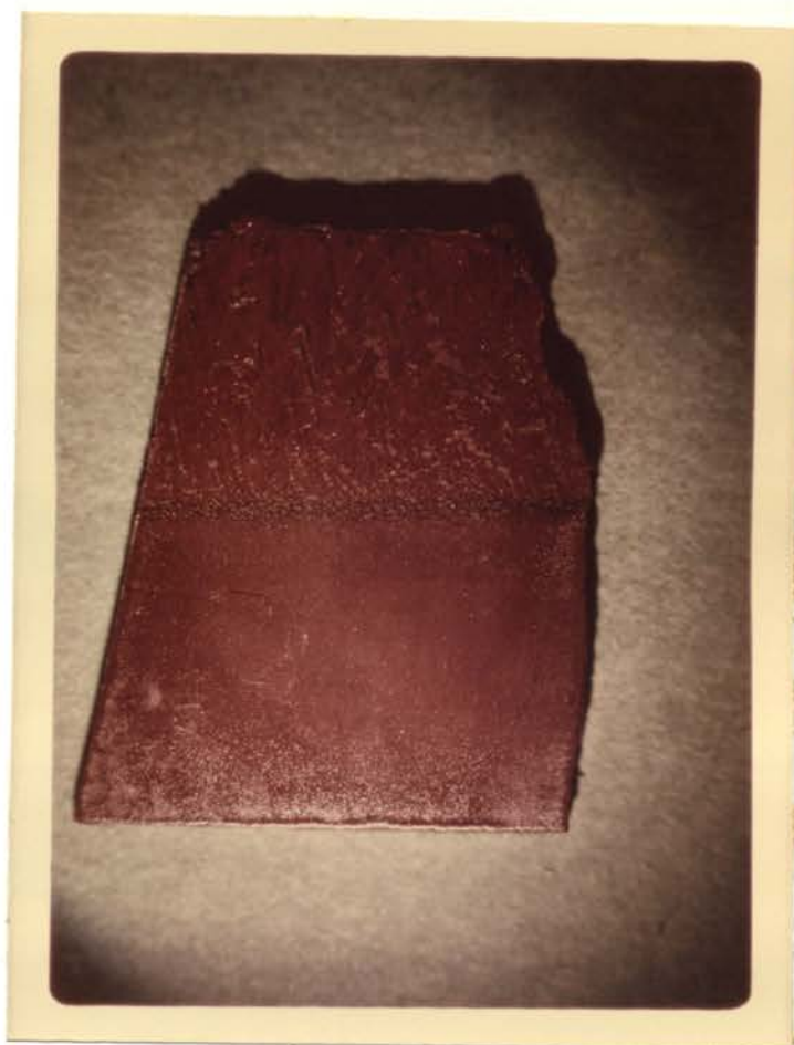
Fig. 48. Polished slab showing cone-in-cone structure. Specimen has been stained with alizarin red S (red areas-indicating calcite) and potassium ferricyanide (blue zone through center of specimen-indicating ferroan calcite). Specimen is from the Dundee Quarry (CDH # 76, L-2). X2.
