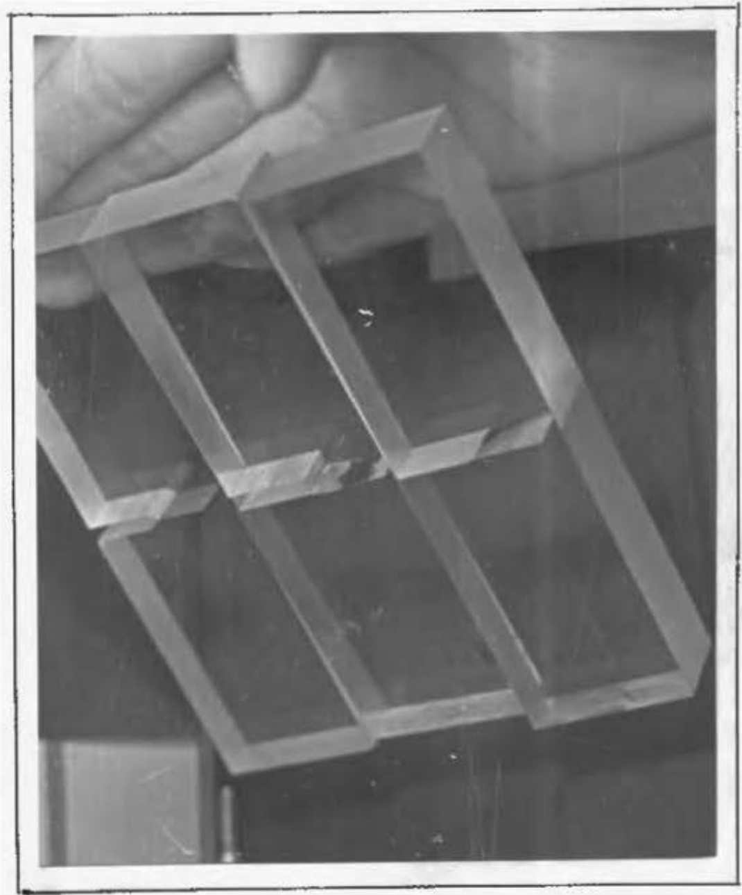
Figure 25. Fracture surface for different types of notch shapes
