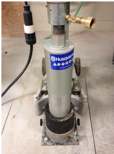
Figure 2 - Specimen Secured in Bottom Jig
