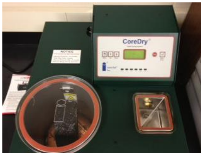
Figure 3.34 - CoreDry Vacuum Chamber
