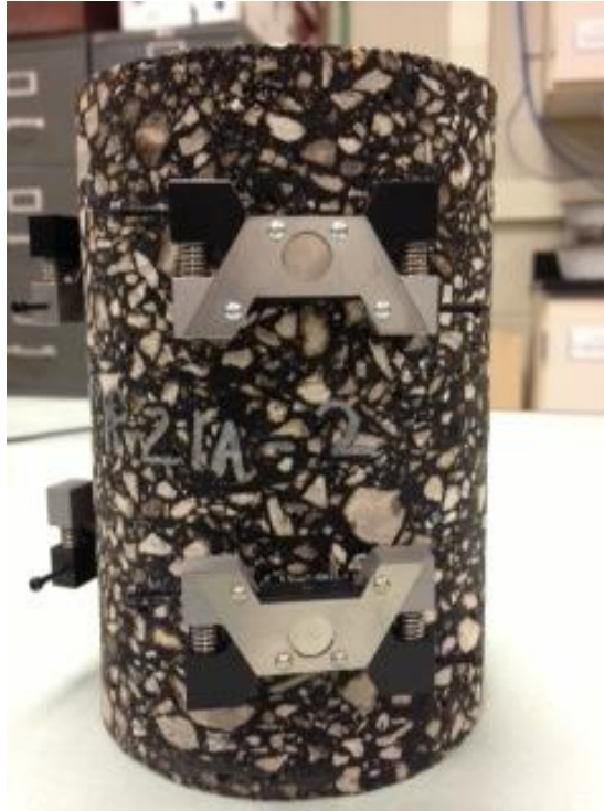
Figure 6 - Clips attached to Gauge Points
