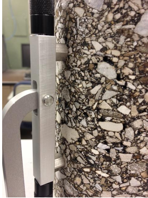
Figure 3.49 – Gauge Points Attached on Specimen Side
