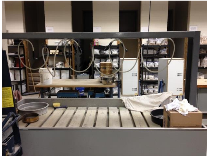
Figure 3.1 - Aggregate Washing Table
