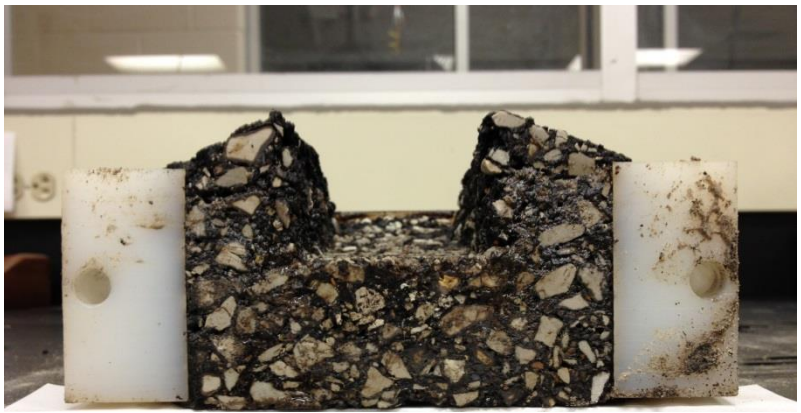
Figure 3.44 - APA Hamburg Test Specimens
