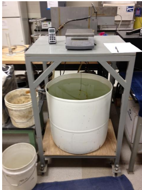
Figure 3.7 - Specific Gravity Weigh-Below Setup
