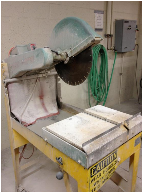
Figure 3.17 - Specimen Wet Saw
