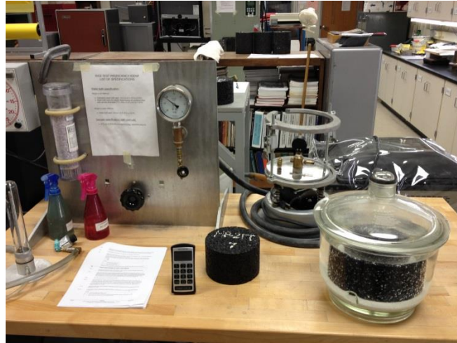
Figure 3.41 - Vacuum Saturation Setup
