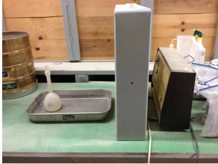
Figure 3.3 - Fine Aggregate Specific Gravity and Absorption Setup
