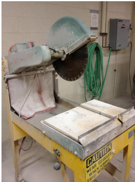
Figure 1 - Wet Saw with Diamond Cutting Blade
