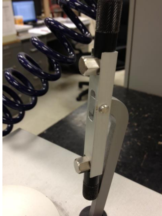
Figure 1 - Fixing Jig Arm with Gauge Points Secured
