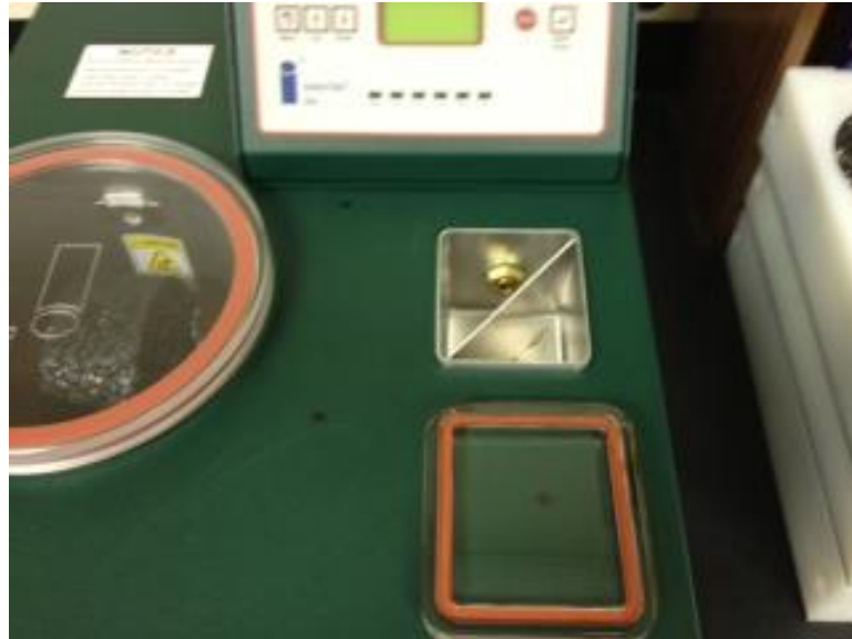
Figure 2 – Cold Trap Chamber with Divider
