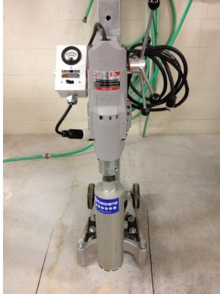
Figure 3.16 - Milwaukee Dymodrill Coring Drill
