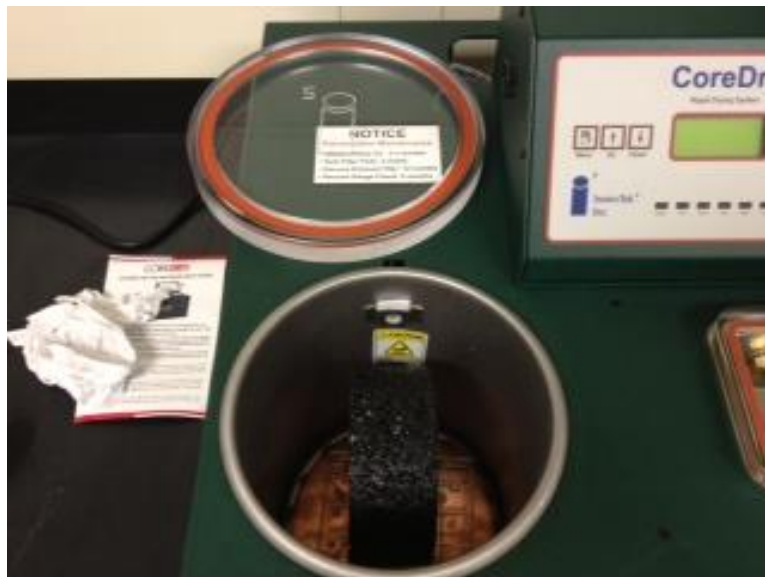
Figure 1 – Vacuum Chamber with Specimen
