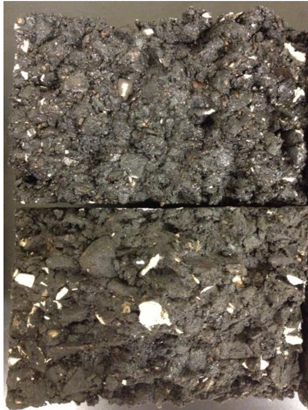
Figure 4.10 – JCD-12 Unconditioned Top/Conditioned Bottom
