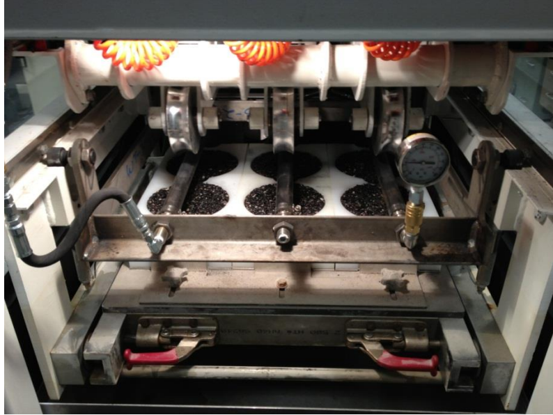
Figure 3.20 - APA Rut Test Setup
