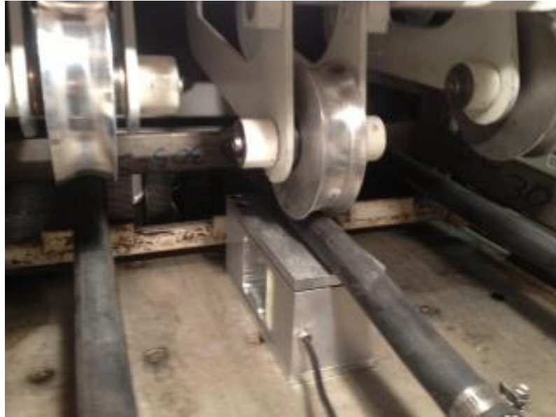
Figure 4 – Load Cell Under Wheel
