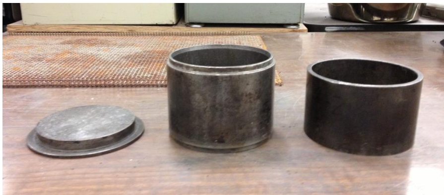
Figure 1 – Base Plate, Forming Mold, & Top Extension Collar
