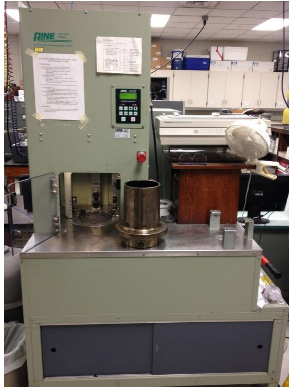
Figure 3.36 - Pine Gyrotory Compactor
