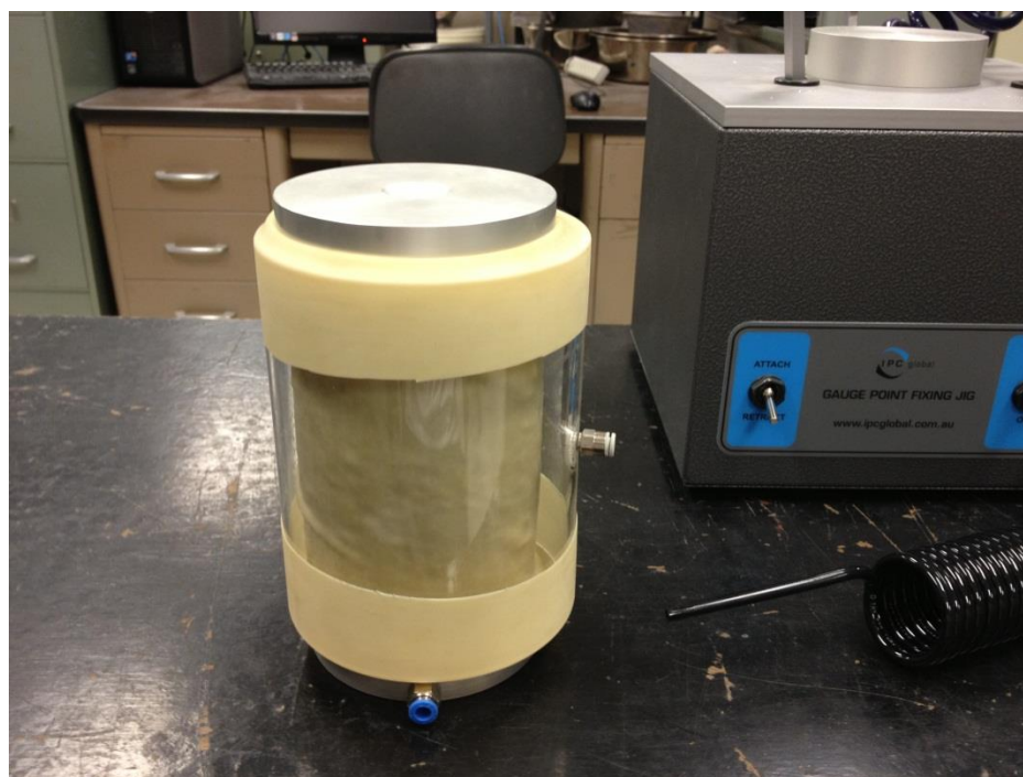
Figure 2 – Collar/Membrane Over Specimen with Vacuum Released
