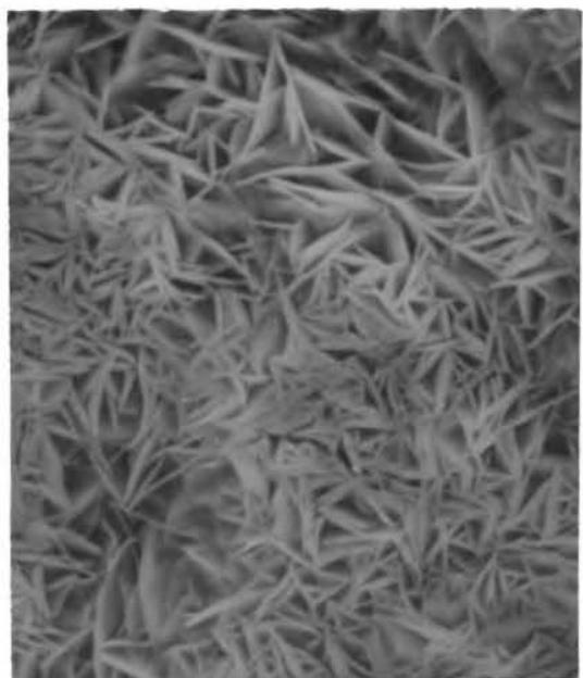
Fig. 53 - Plant Deposit, 3,000X
