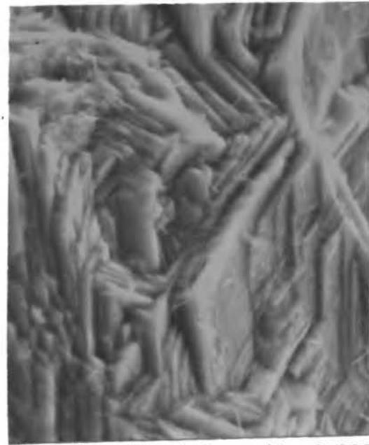
Fig. 50 - Plant Deposit, 3,000X
