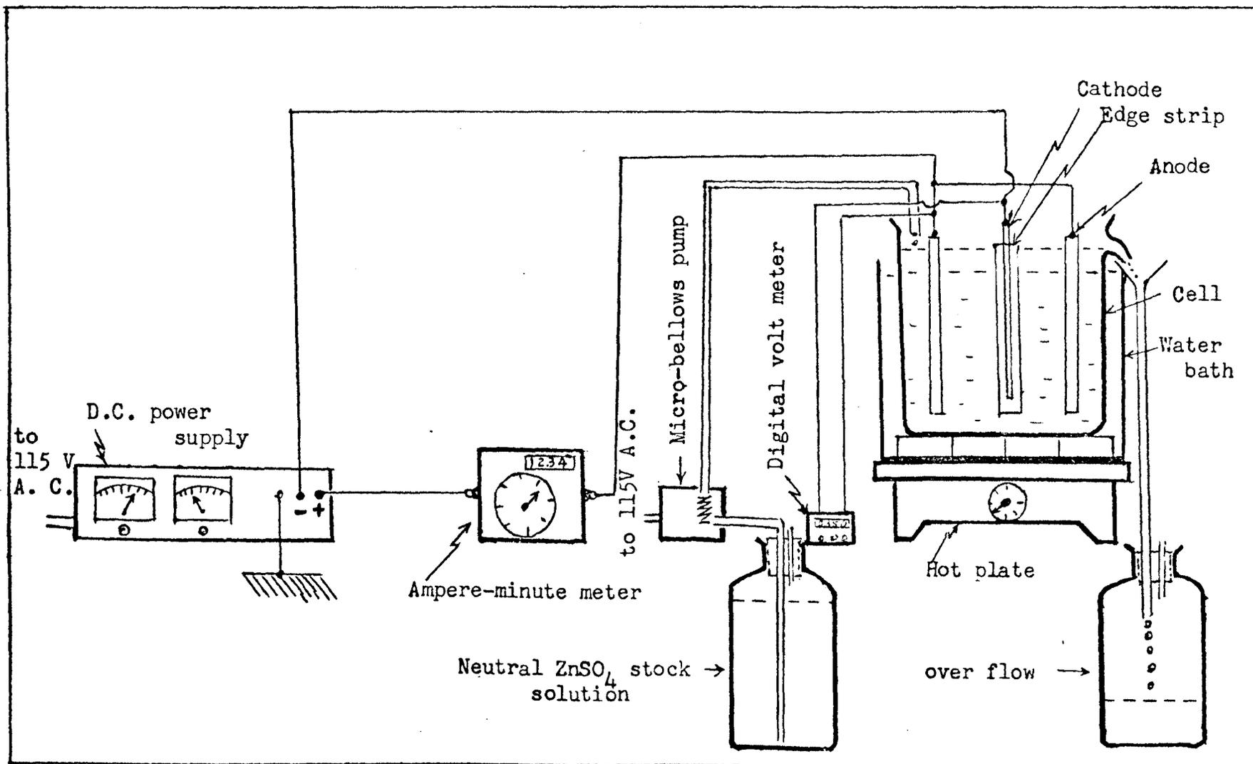
Fig. 3 - Sketch of the experimental apparatus.
