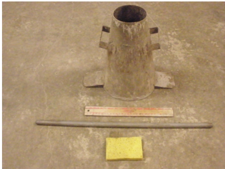
Figure 3.2. Slump Testing Equipment
