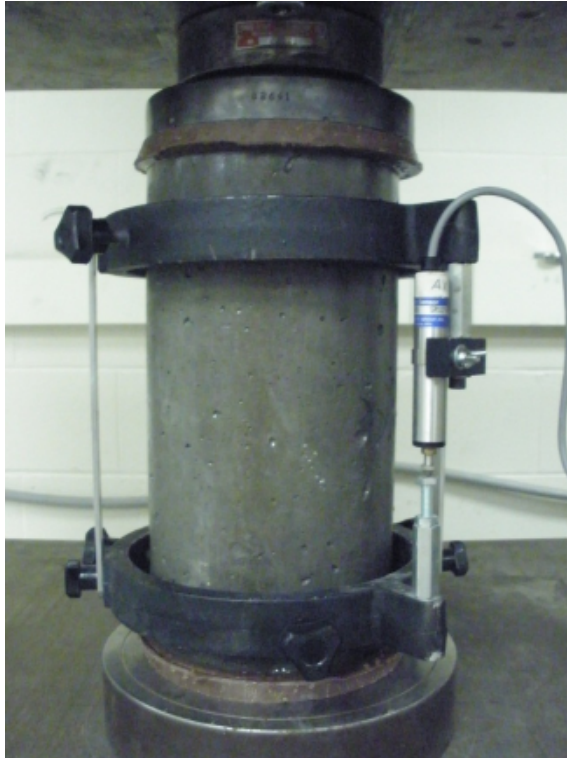
Figure 3.8. Modulus of Elasticity Test Setup
