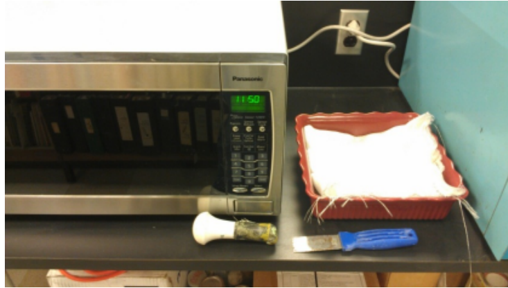
Figure 3.4. Microwave Water Content Station
