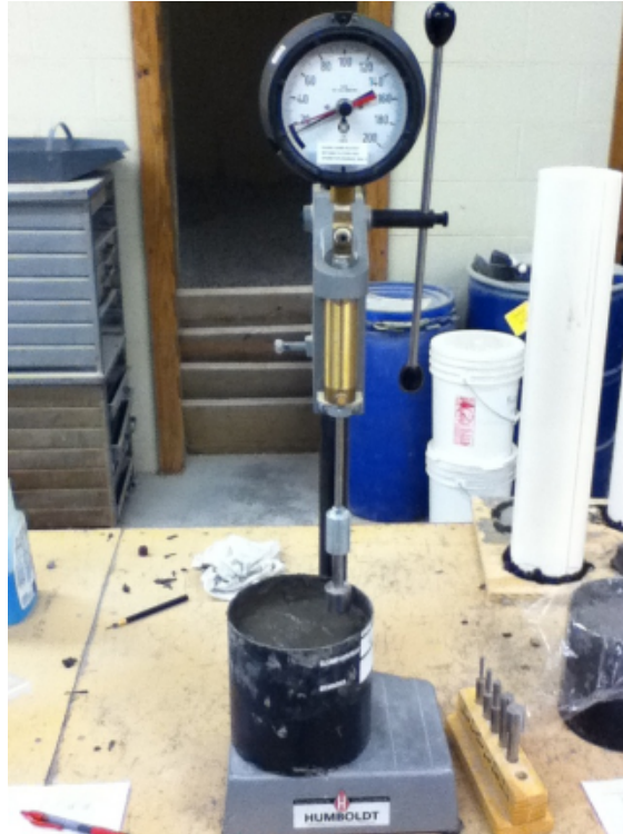
Figure 3.5. Concrete Time of Set Setup
