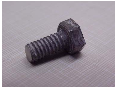
Figure 5: Metal casting of a bolt.
