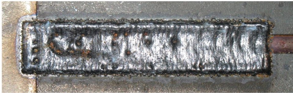
Figure 3: Embedded K-type thermocouple.
