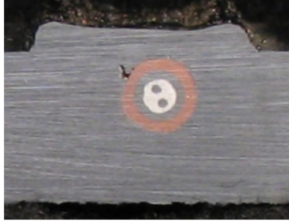
Figure 4: Cross section of embedded K-type thermocouple.
