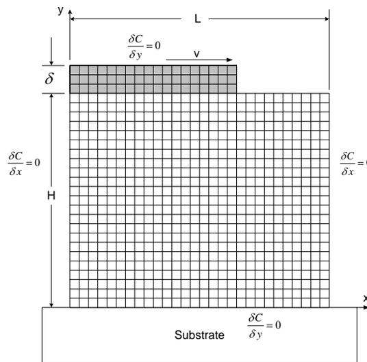
Figure 5: Concentration model mesh and boundary conditions
