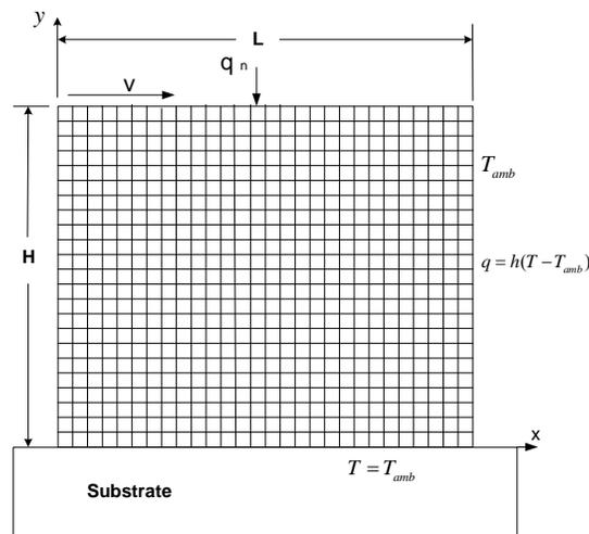
Figure 4: Schematic of semi-empirical thin wall temperature model
